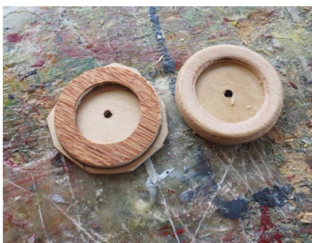
The wheels were a problem, and were made from plywood discs.
