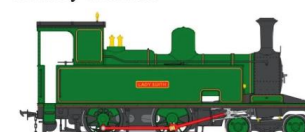
1:20.3 'KATHLEEN' & 'LADY EDITH' Cavan & Leitrim 4-4-0T The model is internally gas fired and has piston valve cylinders. The estimated price is £1950.00 with delivery in 2020
