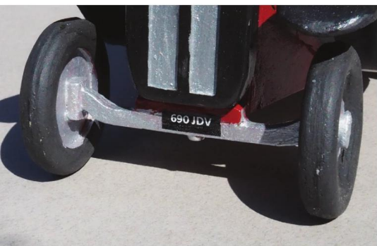
The front axle is cut from 1/8 ply and the dampers are just bits of cocktail stick. The axle is glued on and reinforced with a 2mm bolt self tapped and glued into the ply floor for reinforcement.
