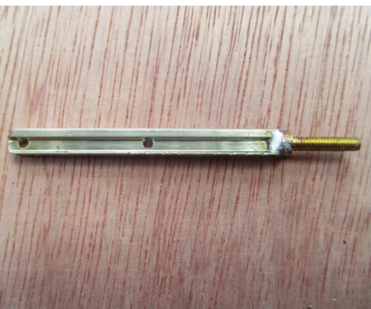
Handrail stanchions were made from some spare lengths of Peco SM32 rail. These stanchions were 2in high and drilled with 2 x 2mm holes to take the horizontal wires. The top end was rounded slightly and the bottom end filed to produce a tongue that fitted into the slot of a brass 6BA screw.
