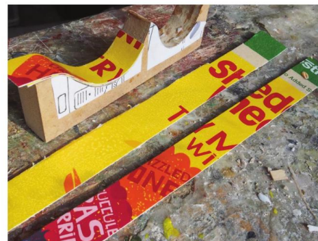
To make the characteristic mudguards I stuck a copy of the drawing onto a piece of scrap MDF and then cut out the shape. The mudguard was then laminated from cereal packet strips glued together with superglue.
