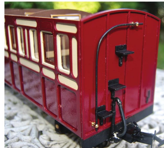
A view of the business end of the coach, the end that the railway staff need access to the roof-mounted compartment lamps. The foot steps came from my spares box, as did the lamp bracket. Roundhouse hand rail knobs and a piece of copper mains wire form the handrail. Vacuum stand with flexible pipe complete the fittings.
