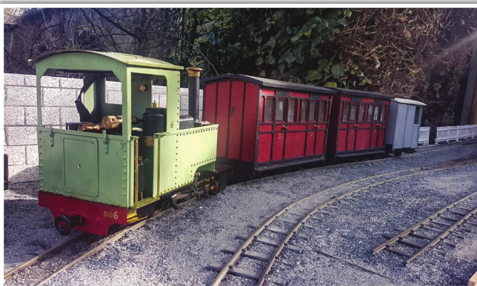
A nice shot of No 6 with passenger stock at Shardlow Road. The coaches and Break Van are built from IP Engineering kits, pimped somewhat. The fencing in the right of the picture is from North Pilton Works, the ballast is Wickes grey paving sand. The walls in the low relief back scene need another coat of Wilko Stone Spray before I coat it with dye brick.
