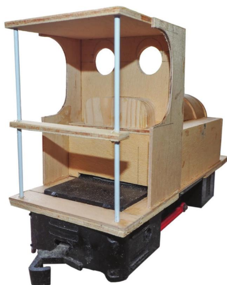
ABOVE: A dummy back-head was made to cover the batteries, then rear cab supports were cut from a coat hanger to create a charming Colonial look.
