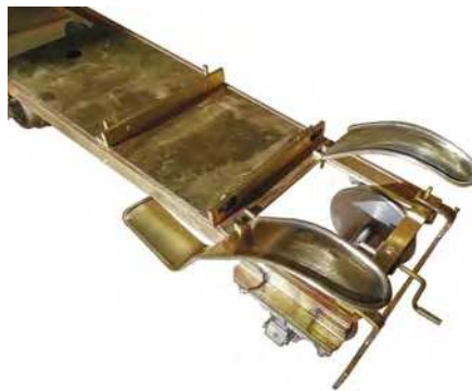
The most difficult part of the construction, forming the wings. This is one area where metal scores over other materials. As well as being the right thickness, it holds a curve so the beading can be fitted to the edges. Axlebox castings are from IP Engineering.
