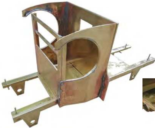
Soldering the bodywork is challenging because the large areas of metal act as a heat-sink. A small gas torch is useful for the job.
