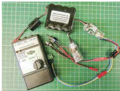
The Fosworks radio control system pre-assembled on the bench for testing before fitting to the model. In the centre of the photo we have the receiver, above this the battery pack and on the right, the speed control.
