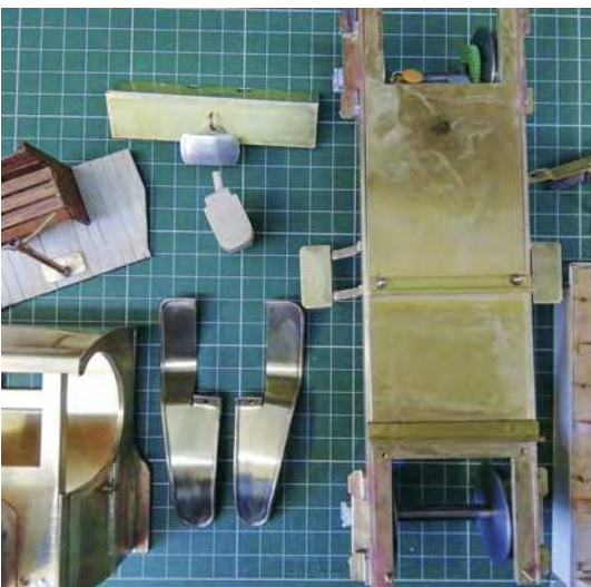
All the components are bolted together, making it easy to dismantle the model for painting.
