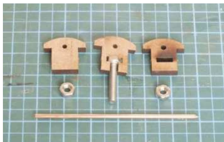
The parts of the buffers, the most ingenious part of this kit.
