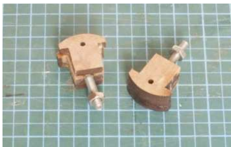
The left hand side buffer is shown not glued to illustrate the assembly process. The right one is completed.
