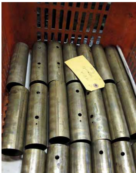
A tray of Mamod rolled boilers awaiting the next stage of the process that will turn them in to pressure vessels.
