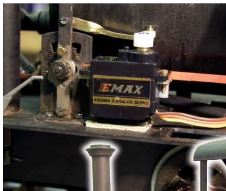
The replacement, larger reverser servo.
