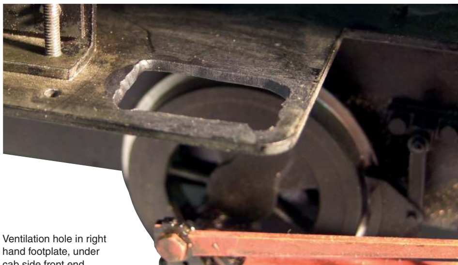
Right hand cab side, showing extra ventilation hole.
