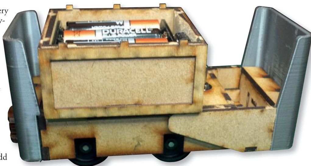
The location of the battery box. The prototype had a step between this and the front end of the loco. This will be modelled later.
