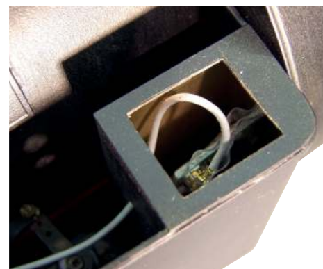
Right: Receiver fitted inside the right-hand cabside 'pocket'. Note aerial passing through hole in rear.
