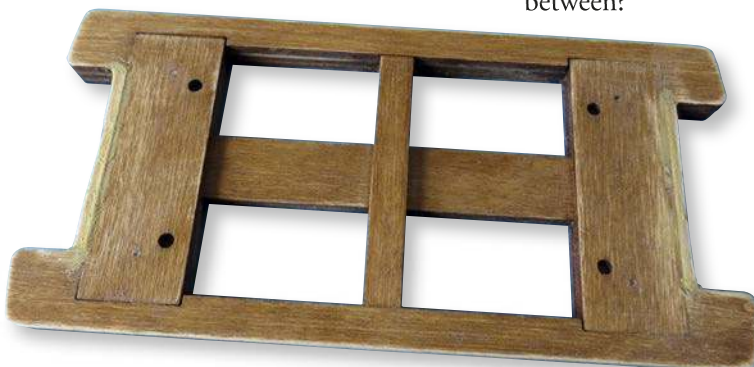
Chassis with the modelling filler applied to the unwanted join lines. It now needs sanding off ready for paint.
