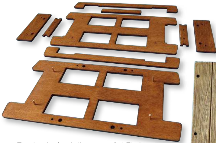
The chassis after shellac was applied. The brass pins that make the alignment of the parts easy can be seen located in the laser cut holes.
