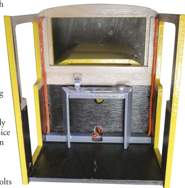
Additional window frame, plus the slightly altered and enhanced control panel. The bare ended wires to left and right supply the roof lights.
