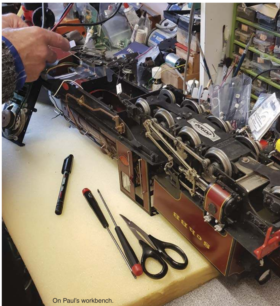
The chassis striped down showing corrosion behind the wheels.
