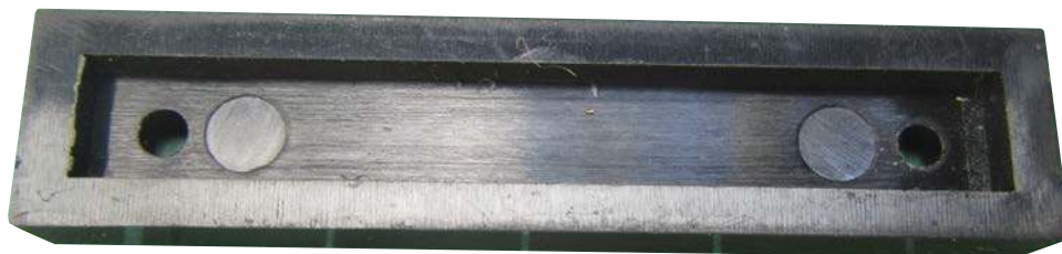
This spacer piece was removed from under the 'W' irons.
