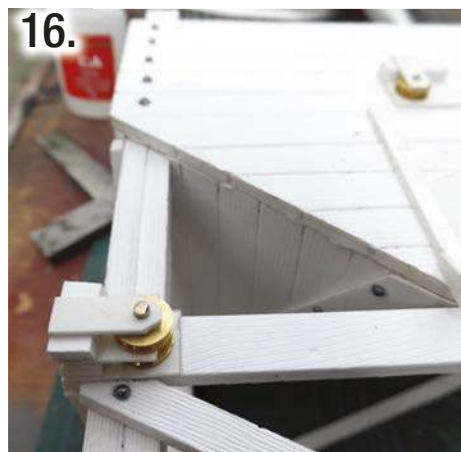
16. The double pulley block was fixed in place on one of the front legs.
