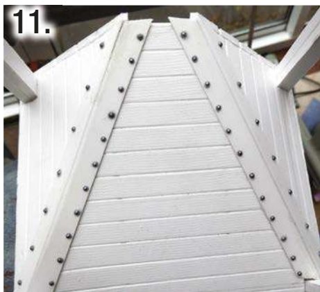
11. 10mm wide strips of 1.5mm thick Plastikard were glued to the lower angled corners of the hoppers and to the vertical corners. 2mm diameter half-round nail art gems (from eBay) were then glued to coincide with the planking representing bolt heads.
