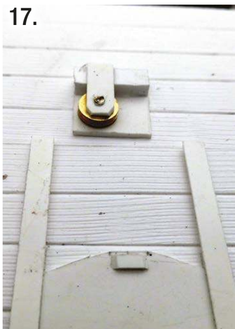
17. The single pulley block was glued above the middle of the sliding door.
