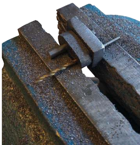
Above: Profiling the cranks to a template.
