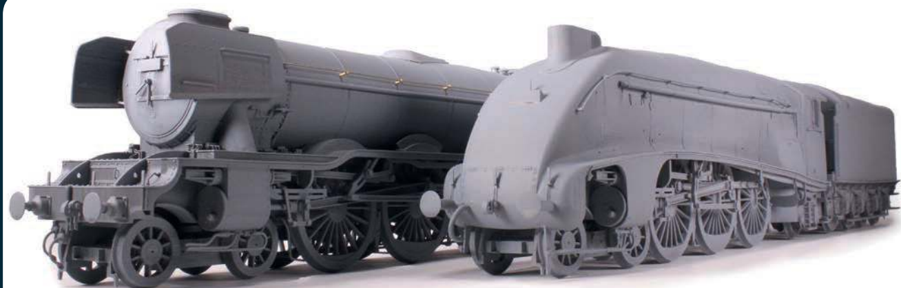
3D printed samples shown
