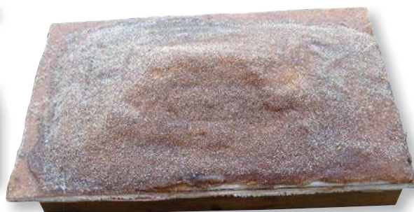
The upper side of a sand load insert. These are removable so the wagons can run as empties Down the line.
