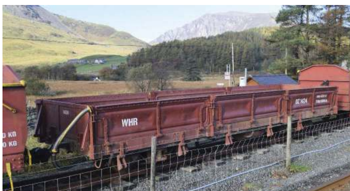
Type DZ low-sided ballast wagon, modified with removable ends. (Photo: David Williams)
