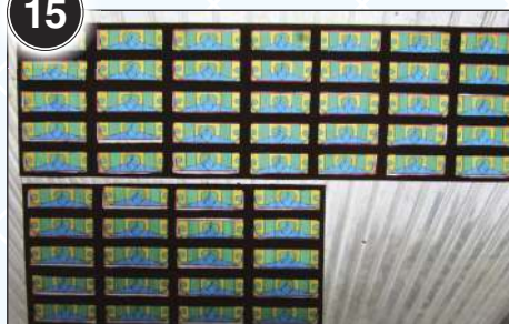
The frames were glued to one side of a sheet of 2mm thick clear acetate (using clear Bostik) and the printed overlays glued to the other side.
