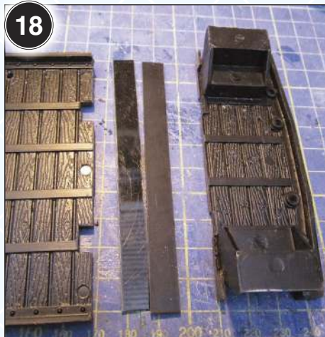
The frames were glued to one side of a sheet of 2mm thick clear acetate (using clear Bostik) and the printed overlays glued to the other side.
