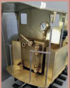
Hidden burner in the cab
