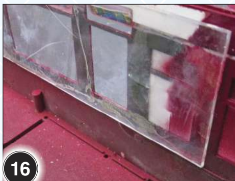
A couple of strips of the 2mm thick acetate were glued behind the window frames on the coach body.
