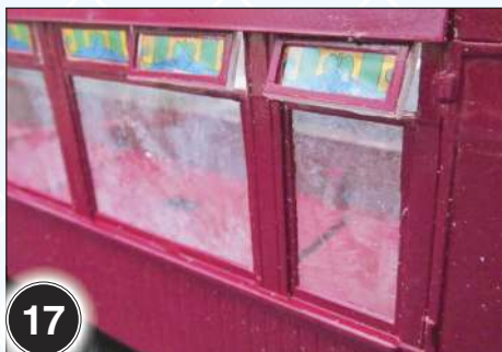
The frames were then cut out from the acetate and glued into toplight openings. Some in the open position and some in the closed position.
