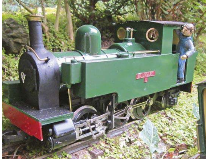
Former Southwold Railway Sharp Stewart No. 1 (Southwold) re-imagined with a scratchbuilt body on a Playmobil 0-4-0 motor block. Its MyLocoSound sound card is housed in the bunker. The majority of my locos now have soundcards.
