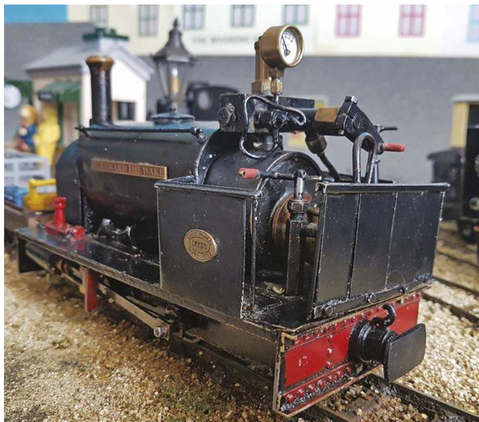
Close-up of port stern – cab much clearer now, the pipework is still a bit baroque, but plumbed into the steam turret
