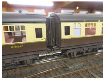
Magnetic coupling corridor connections
