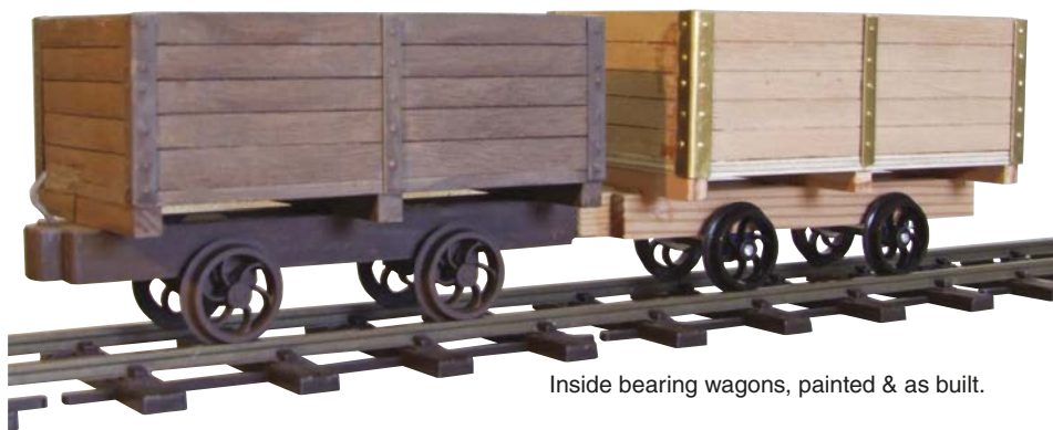
Miniature railway wagon before conversion (right) & after (left).
