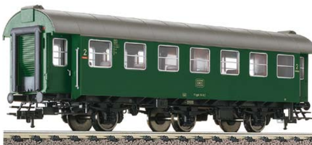
2nd class, 3-axled coach, type B3yg 761, of the DB. 2nd class, 3-axled coach, type B3yg 761, of the DB.
