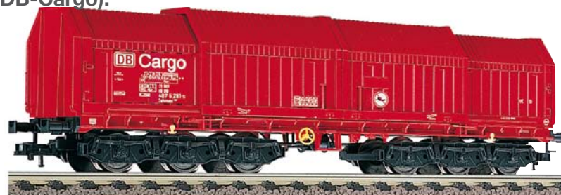
Telescopic sliding cover wagon, type Sahimms 900, of the DB AG (DB-Cargo).
