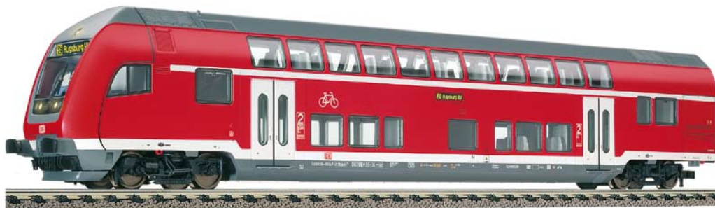
2nd class double-deck control-cab coach, type DBpbzfa 766, of the DB AG.
