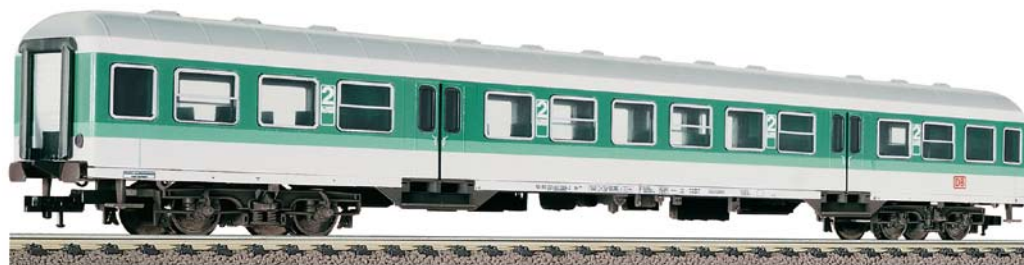
2nd class control-cab local coach, with bicycle compartment, type Bnrdzf 477, of the DB AG.
