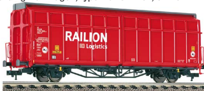
Sliding wall wagon, type Hbins-tt 292, of the DB AG („RAILION“).
