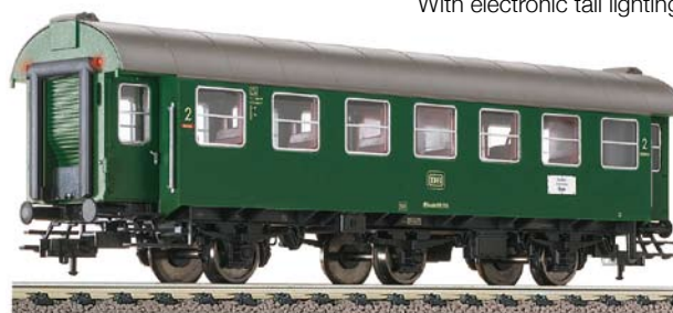
2nd class, 3-axled coach, type B3yg 761, of the DB. 2nd class, 3-axled coach, type B3yg 761, of the DB.
