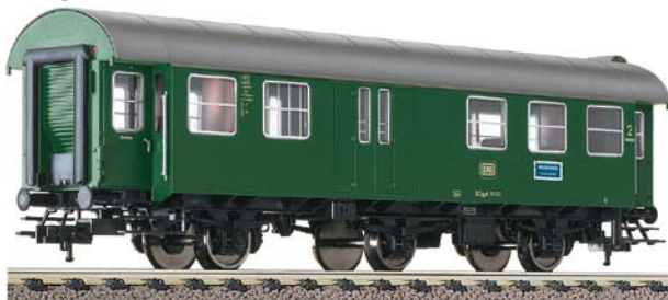
2nd class, 3-axled coach with baggage compartment, type BD3yg 766, of the DB.
