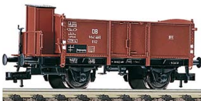
Lidded wagon with brakeman's platform, type K 15, of the DB.
