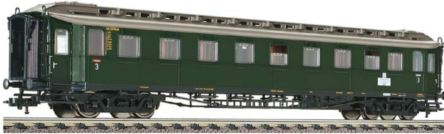
4-axled, 3rd class coach, type C 4ü (Pr08), of the DB, with tail indicators.
