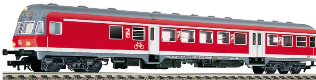
2nd class control-cab local coach, with bicycle compartment, type Bnrdzf 477, of the DB AG.
