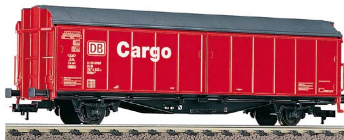
Telescopic sliding cover wagon, type Sahimms 900, of the DB AG (DB-Cargo).
