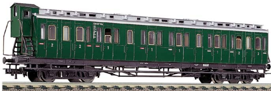
1st/2nd class compartment coach with brakeman's cab, type AB4 (BCpr04), of the DB.
