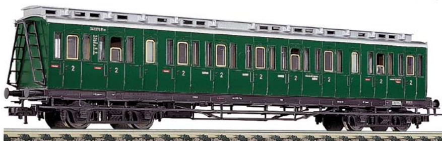
1st/2nd class compartment coach with brakeman's cab, type AB4 (BCpr04), of the DB.
