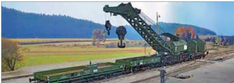
R-02: KM1 90-Tonnen- Kran in 1
