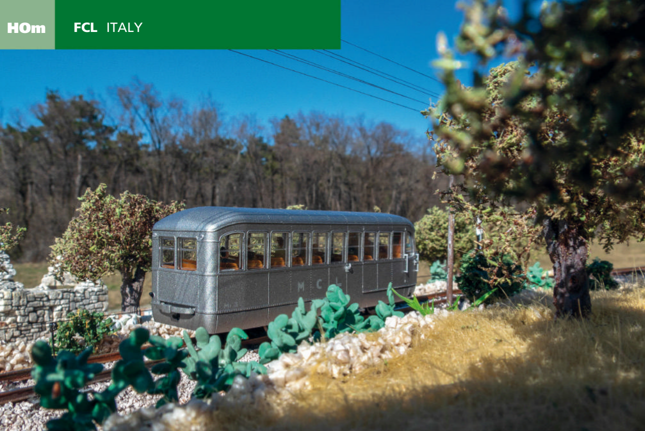
Left M1.3 climbs the gradient between the dry stone walls and the prickly pears that border the olive groves. The Emmine were single cab railcars very similar to buses. At termini it was necessary to turn them by hand on special small turntables.
