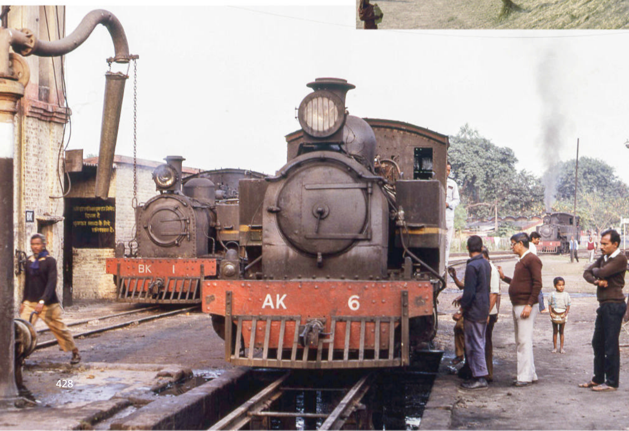
Below Katwa shed, with Bagnall 0-6-4Ts BK1 (2006 of 1914), AK6 (2021 of 1916) just arrived from Ahmadpur, and beyond BK4 (2009 of 1914) preparing to take the next train to Ahmadpur. Although nominally allocated to Ahmadpur – Katwa (AK) and Burdwan – Katwa (BK), the locos worked either line.
