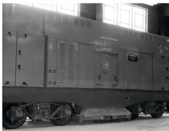
Right Part of one of the filter cars, on standard freight trucks.
