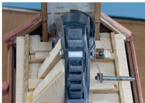
Below right Side view of the top of the mechanism with the gerber in position to discharge into the spout filling the rail car.
