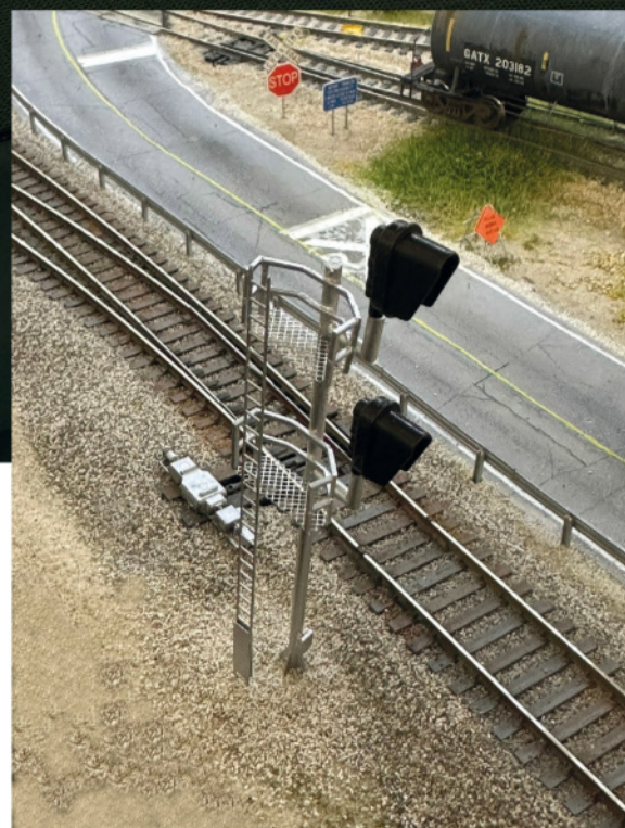
Right One of the scratch-built signals – Plastruct railing, with Walthers chain link fencing panels cut and fitted horizontally to represent metal tread plate, an Eckon ladder, and BLMA (now Atlas) signal heads. These have ready wired LEDs but making them work is way beyond my electronic skills.
