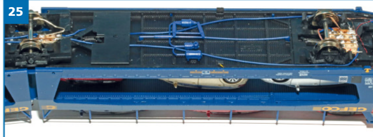
25 The underframe of the half of the wagon with the lamps.
