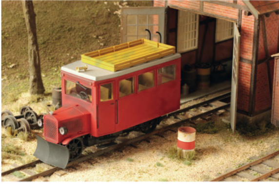
Above This railcar was largely built from 3D-printed parts on a modified Bachmann mechanism, as fully described in the following article.
