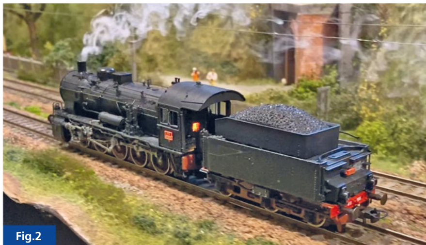
Figure 2 The FS Gr.473 0-10-0 (former Prussian G10) made by Roco in 1983 to which a decoder with loudspeaker was added in the tender (which involved milling the coal), plus a light in the firebox, and modified current pick-up.
