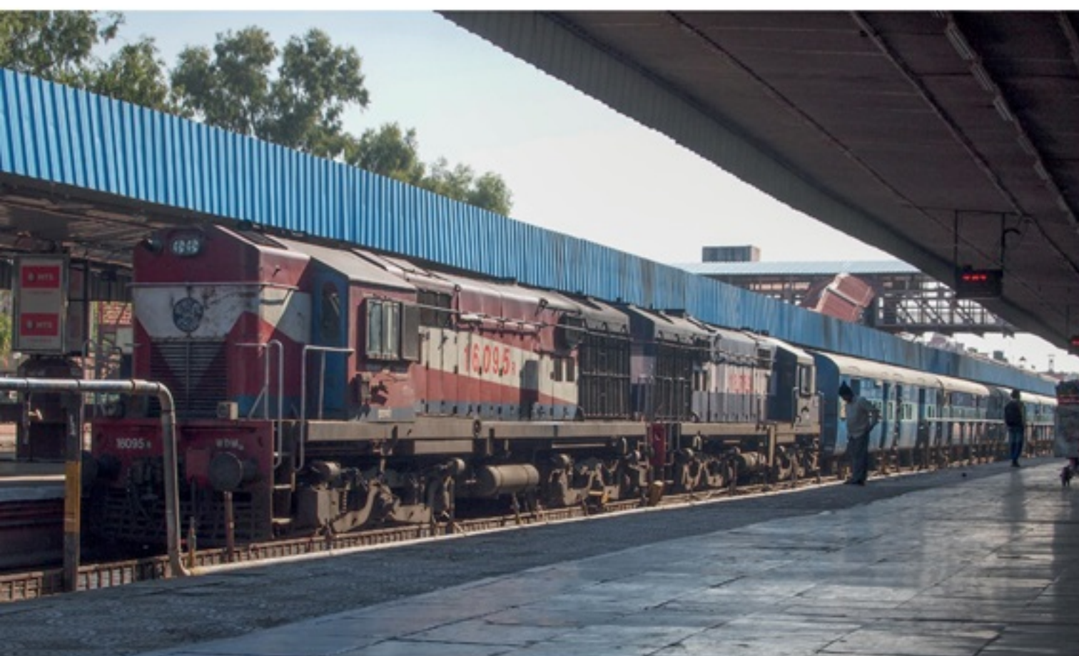
Below A pair of WDG3A diesels banking an express at Jaipur; these trains can be up to 26 coaches.
