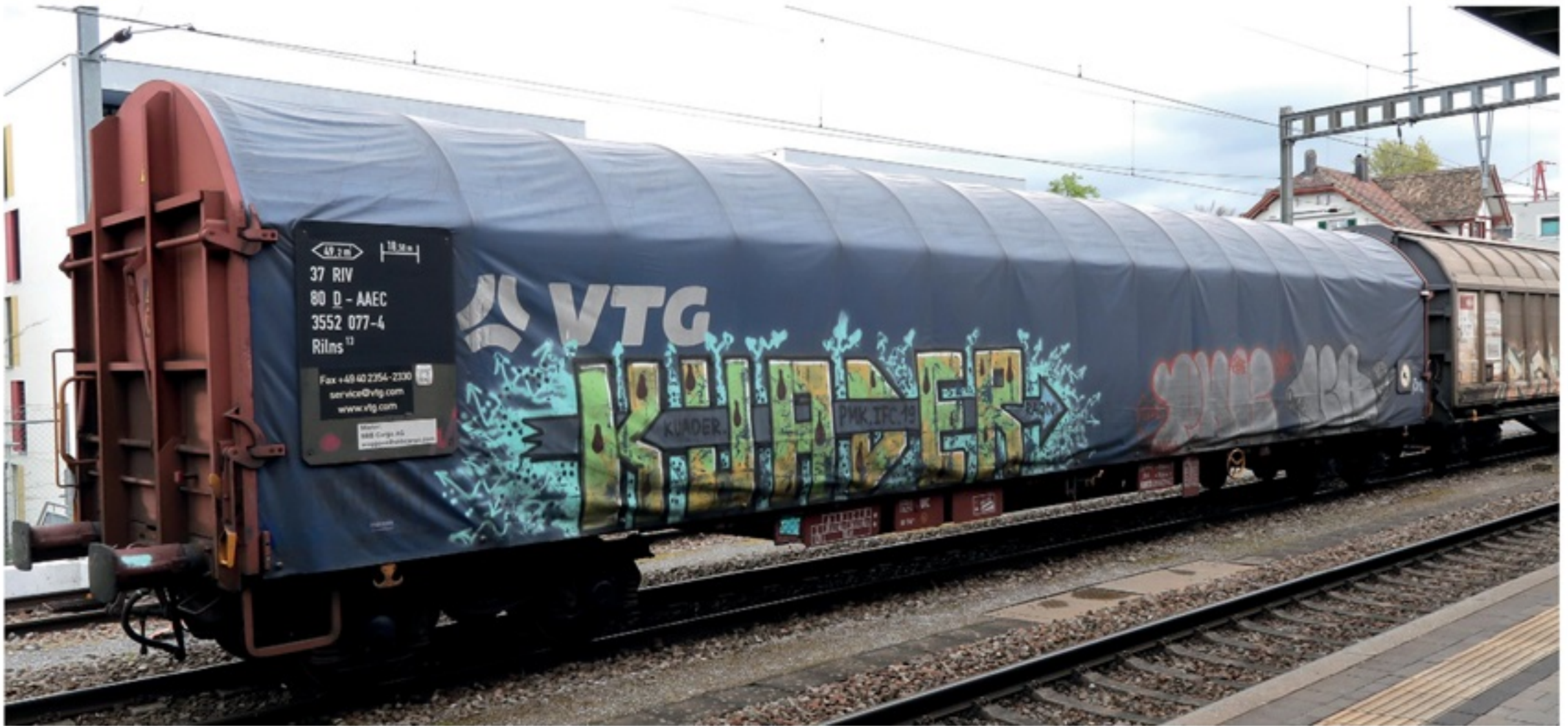
Above VTG Rilns tarpaulin covered bogie bulkhead flat at Frauenfeld, 25th April 2022.
