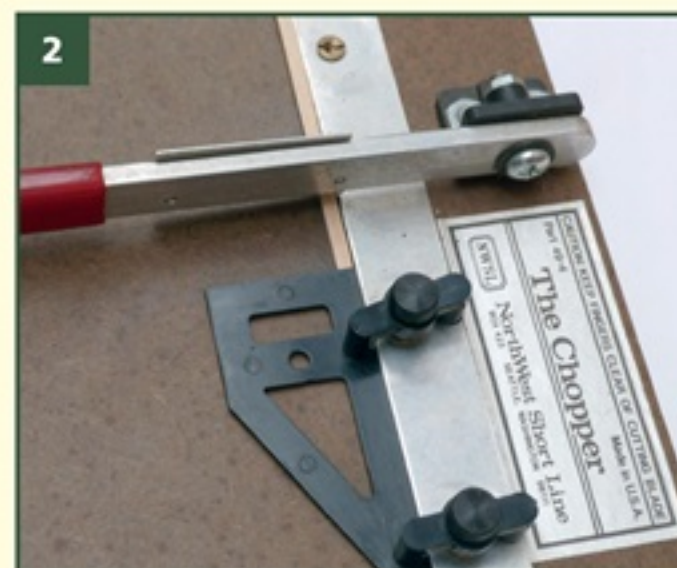
2. The modeller's guillotine used for cutting the endless supply of sleepers to length, squarely. Invaluable.
