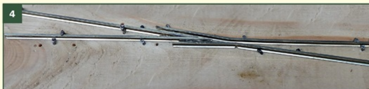
4. The rail components for one of the common crossings, pinned down to the jig prior to soldering.
