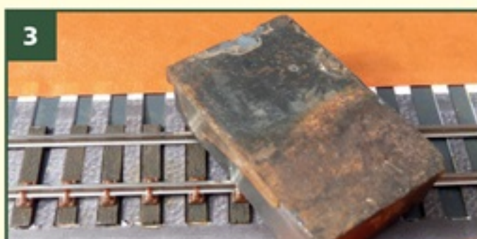
3. The cut-out sleeper spacing template, with the first row of baseplates being held down by a magnet while the glue hardened.
