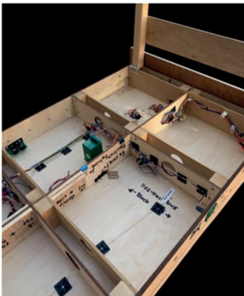
Left The underside of one board, showing the sandwiched beams used to strengthen the base and the hinged legs. Photo: author.
