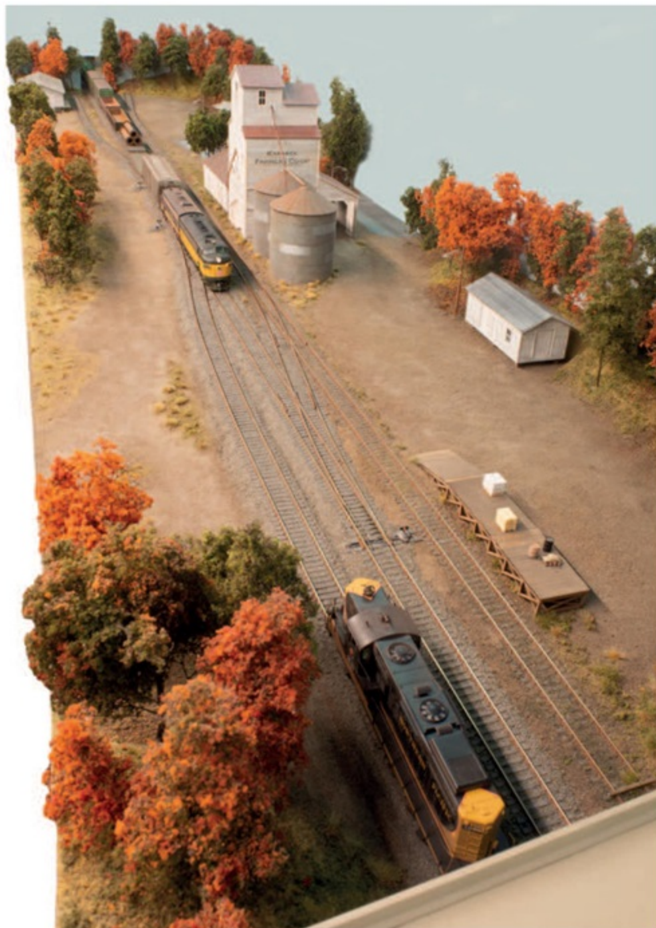
Below One train is held on the passing siding under the road bridge as another rolls by on the main. Spurs serve the team track, the grain elevator, and a warehouse.
