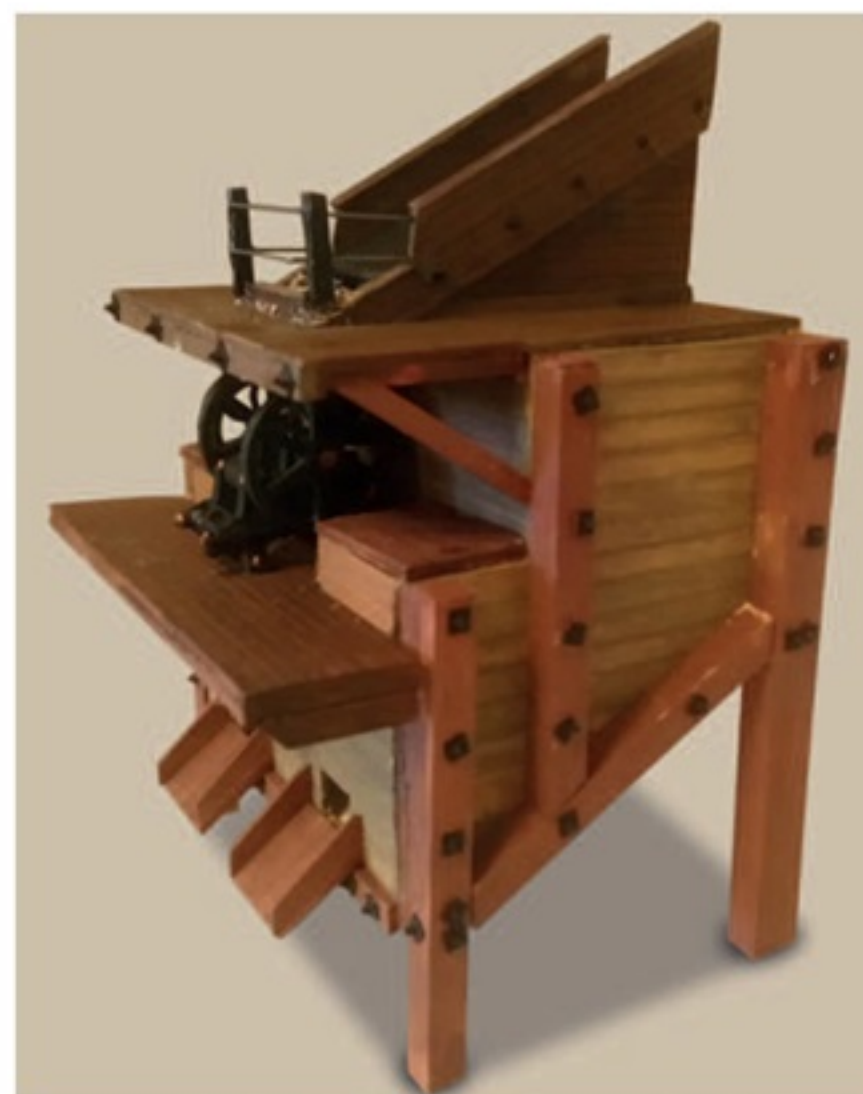
Right Ore bin complete with grizzly, crusher, and chutes.
