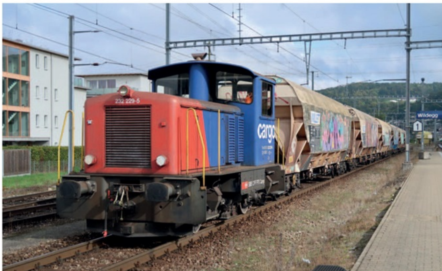
Left and right The Jura Cement factory at Wildegg requires a lot of shunting with Tm 232 tractors. Passing freight services leave wagons for the works in the adjacent loops and a 232 (here 232 229-5) moves them in and out of the factory sidings. 8th October 2021.
