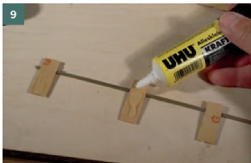
Left After the first rail has been soldered to the spacers, the track is glued to the board and the second rail can then be soldered.
