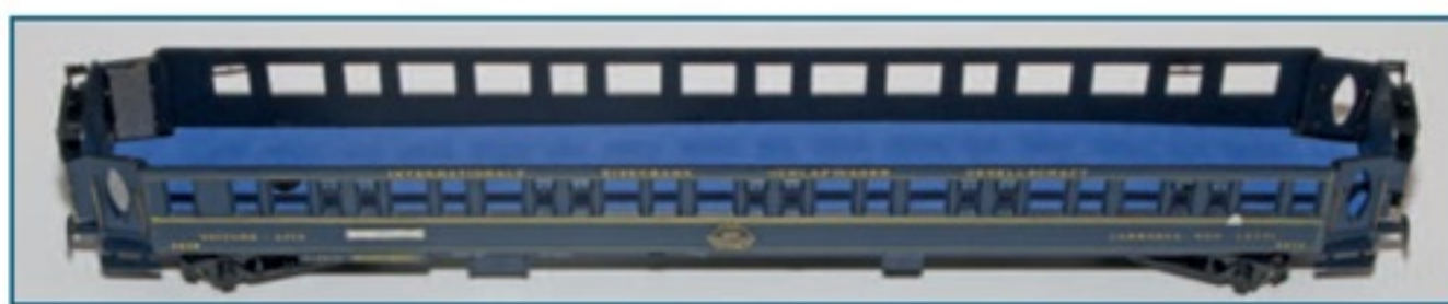
Right The sugar paper was trimmed at the ends to fit inside the car body, with a hole for the pivot.
