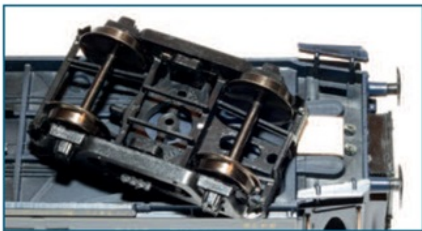
Above To install the SMD coupler pockets, I had to level two small projections under the frame, near the buffer beam, with a piece of plasticard.
