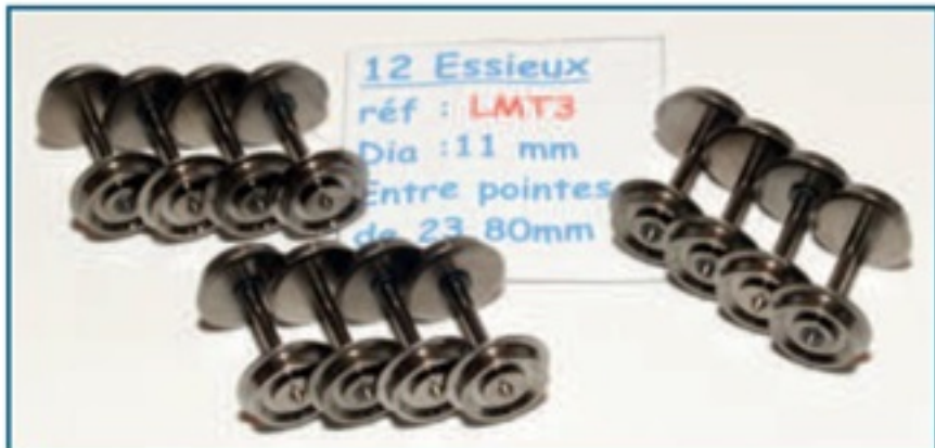
Left I replaced the wheelsets, using 11mm dia. disc wheels on 23.8mm pinpoint axles from Limousin Models (ref.LMT3). These give flawless running and impeccable rail-wheel contact for the lighting.
