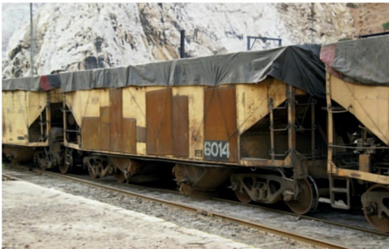
Below This crudely patched FCCA hopper has been put back into service without paint.
