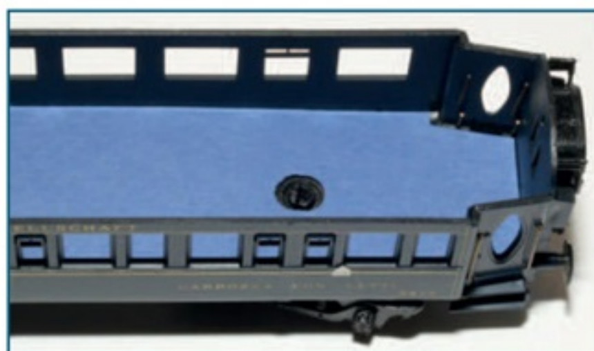
Left I replaced the wheelsets, using 11mm dia. disc wheels on 23.8mm pinpoint axles from Limousin Models (ref.LMT3). These give flawless running and impeccable rail-wheel contact for the lighting.
