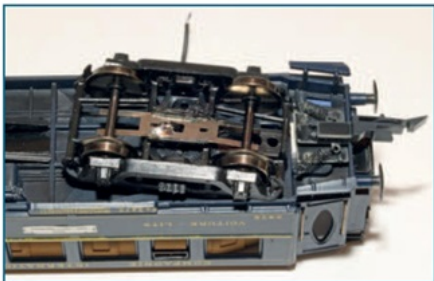
Left Installation of CDF pick-ups under the bogies. The wire has already been soldered to the pick-up; the other end can be seen at the top of the photo: it will be connected to the lighting strip.
