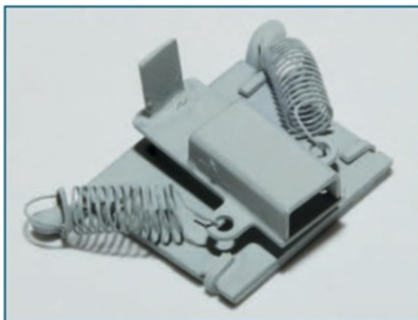
Right An assembled SMD coupler pocket primed with AMF 87 spray paint.
