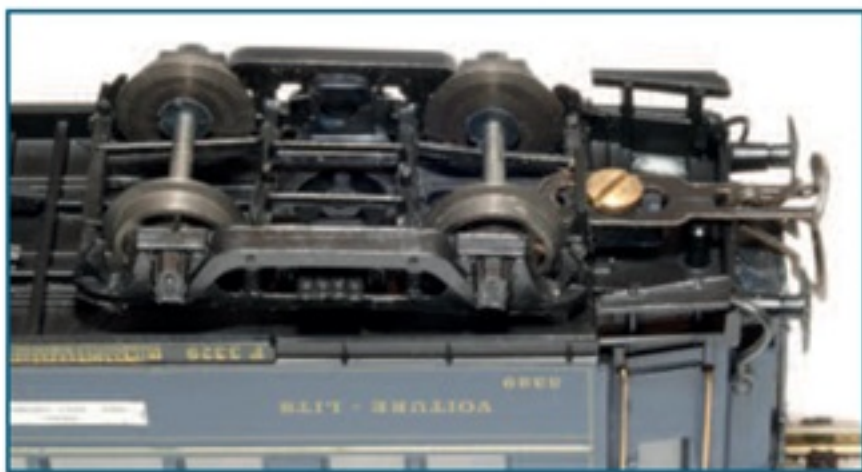
Left Underside of a coach in original configuration.. The buffers are rectangular and have a tendency to lock with those on the adjacent vehicle.
