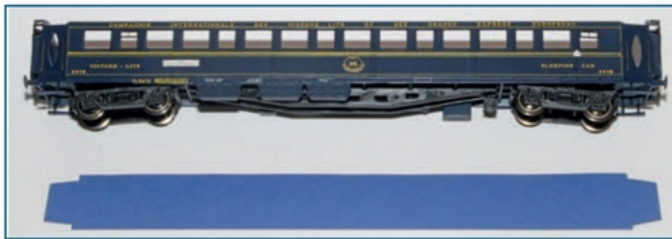
Above and below In some coaches, it may be necessary to place a floor covering cut from blue sugar paper, carefully adjusted at the ends to fit inside the car body.
