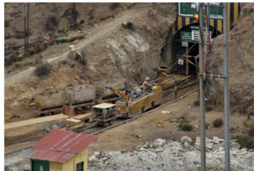
Left and below Numerous mines dot the valley sides. Most of the adits are accessed by narrow gauge lines.
