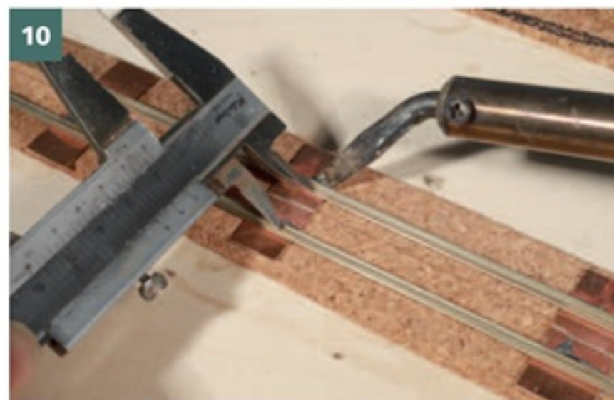
Right The calipers, set to 16.5mm, make an ideal track gauge.
