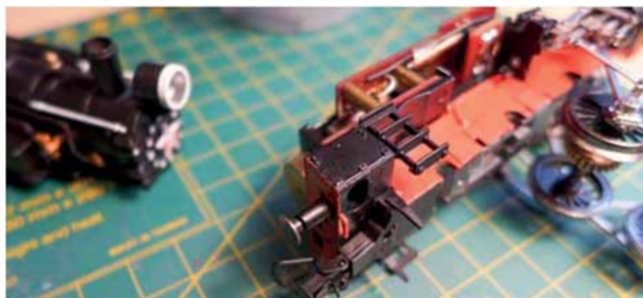
Above Modifications were required to the rear of the chassis removing the air reservoir.
