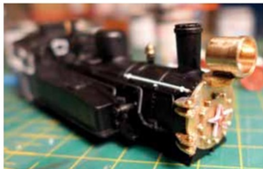
Left Smokebox front in place, held by a projecting pin on the back of the star.
