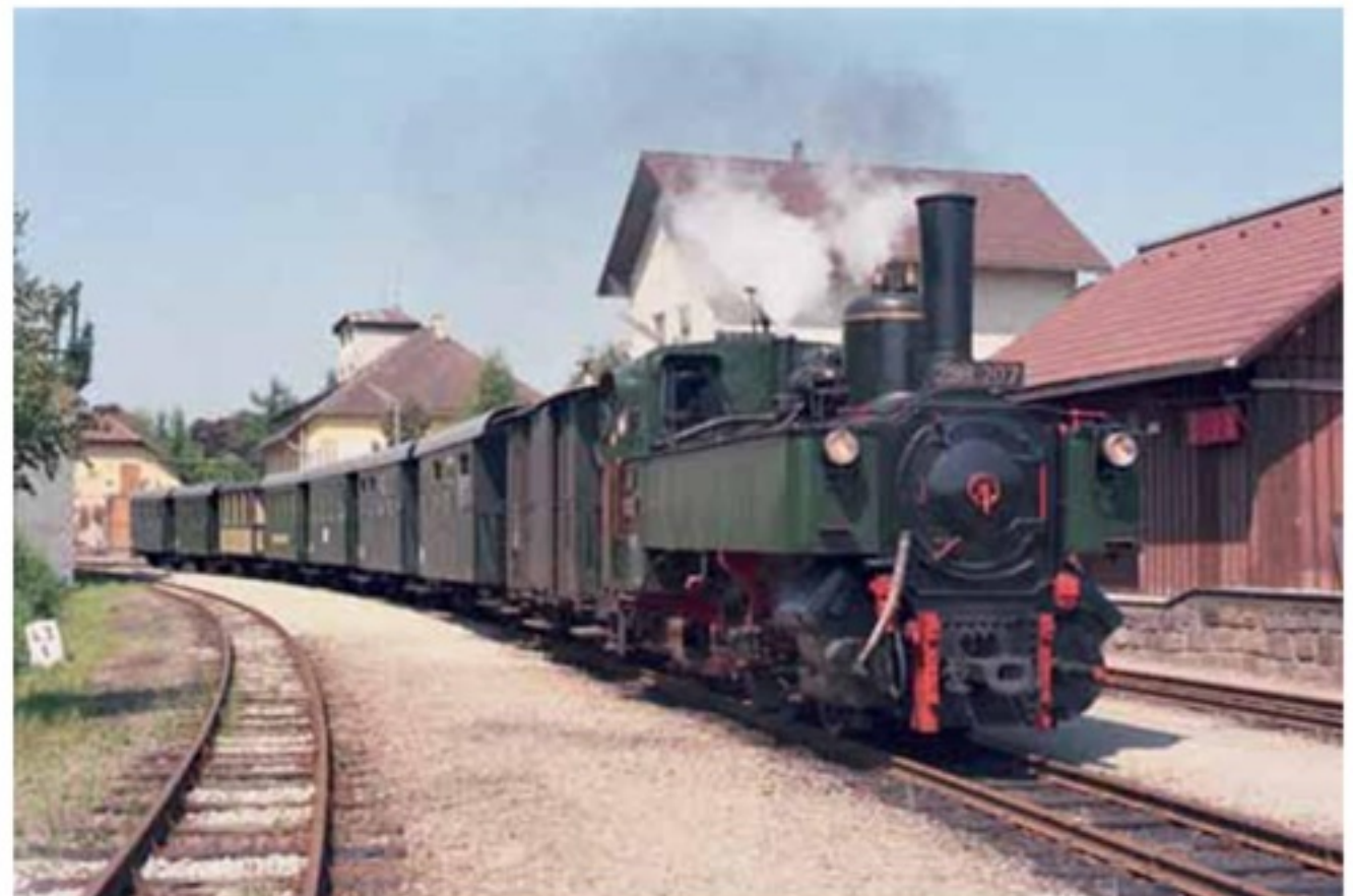
Right 298.207 at Groß Gerungs with the buffet car in the train. This is a Uv class compound – the larger low pressure cylinder is clearly visible on the left-hand side of the loco. June 1987.
