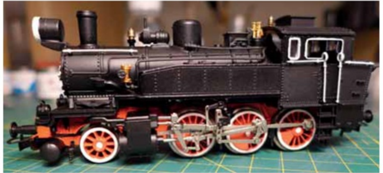
Above Headlight, tyres, handrails and window surrounds are picked out in white.
