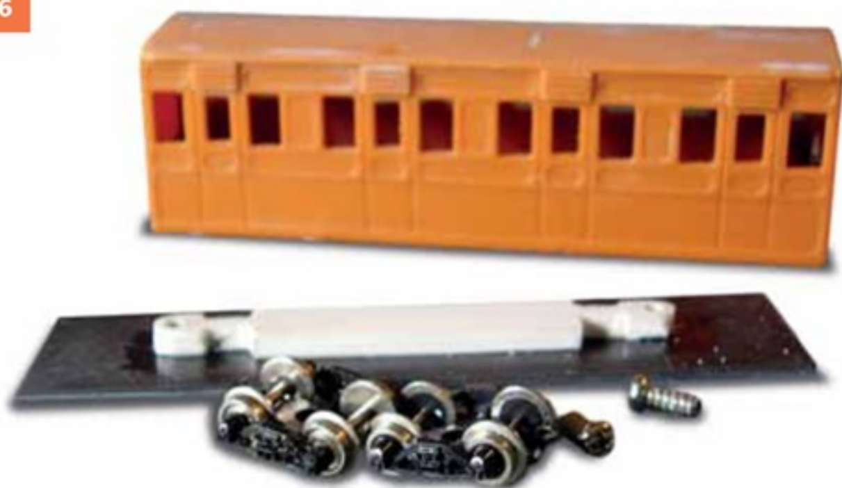
The new underframe starts as a flat strip of plasticard to which a shaped spine and bogie mounting pads assembly is fixed.
