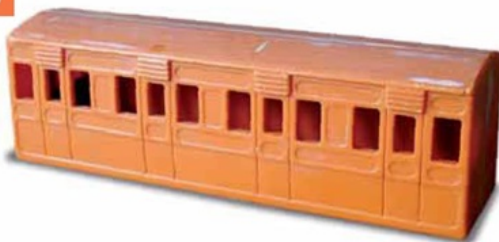
Two applications of filler and lots of sanding later, a smooth arc to the roof is the result.
