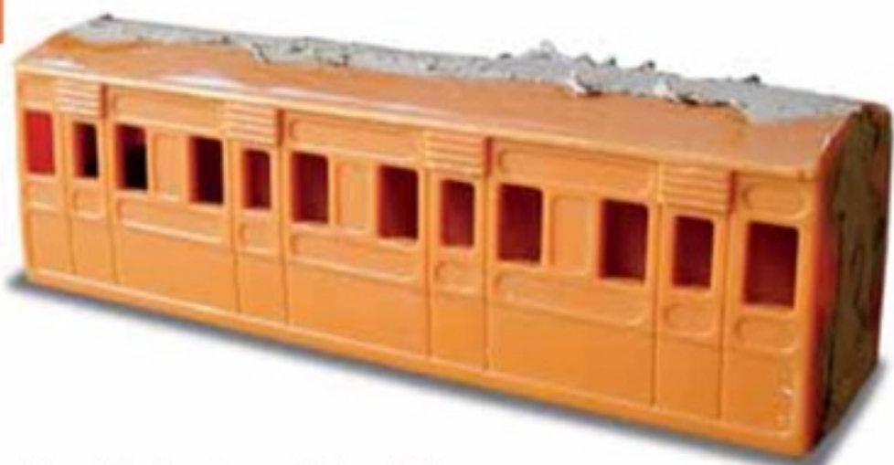
The strangely shaped moulded ventilators have been filed off and filler applied to the gaps in the roof and ends.
