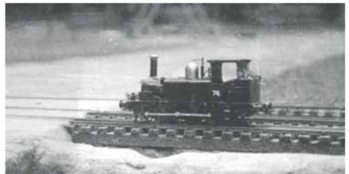
Below Class N67 0-6-0T No.74. Eight copies of Stroudley 'Terriers' were built by local firms (Mort & Company and Vale & Lacy) for suburban passenger work and placed in service in 1875.
