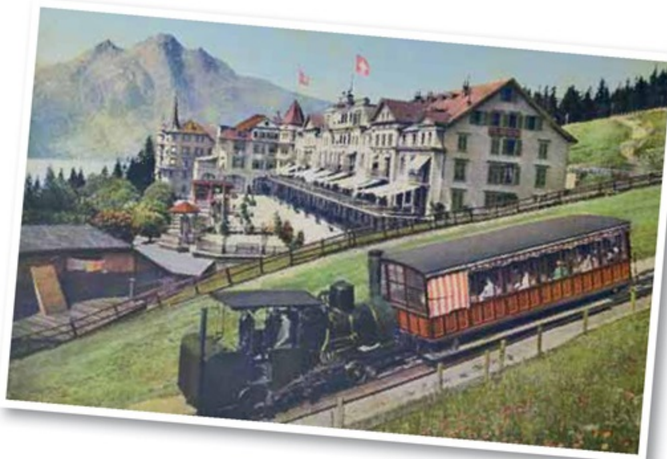
Above A 1920s postcard showing a rebuilt locomotive with a horizontal boiler passing the hotels at Rigi Kaltbad. Photo: author's collection.
