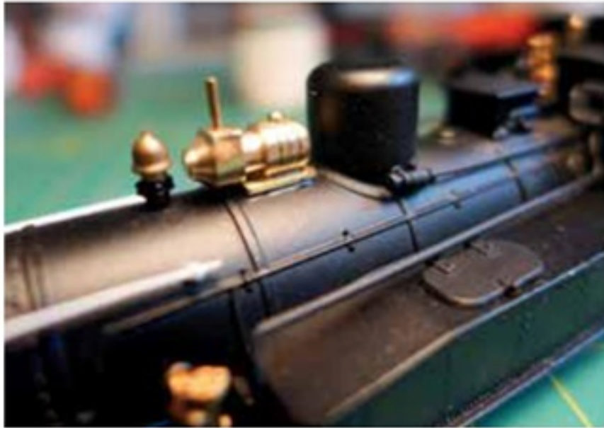
Left The turbo generator was scratchbuilt from brass.
