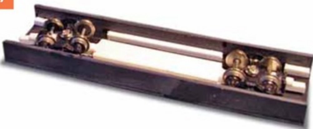
Side sections are added, the corners reinforced and kept at right angles with square section strip.
