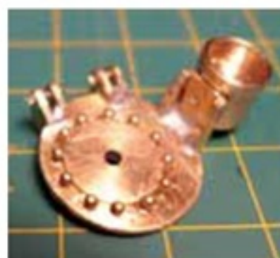
Above The new smokebox front, fabricated with door, clamps, hinges, and headlight.
