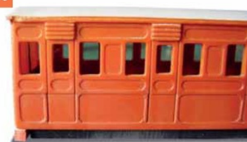
After sanding back the filler, a thin coat of primer reveals promising radiused corners.
