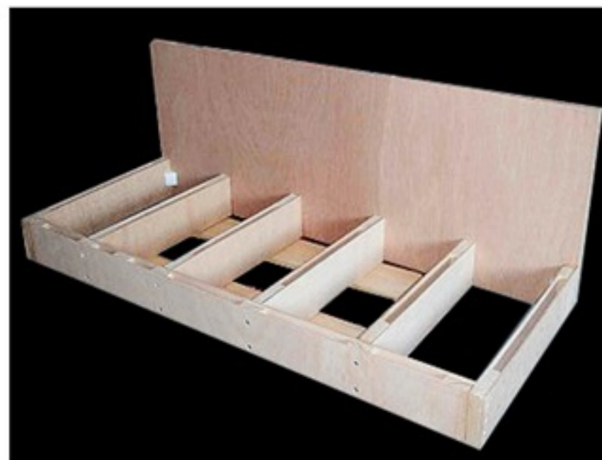
Far left The baseboards were made using sandwiched ply beams with plain flat tops for the storage yard.
