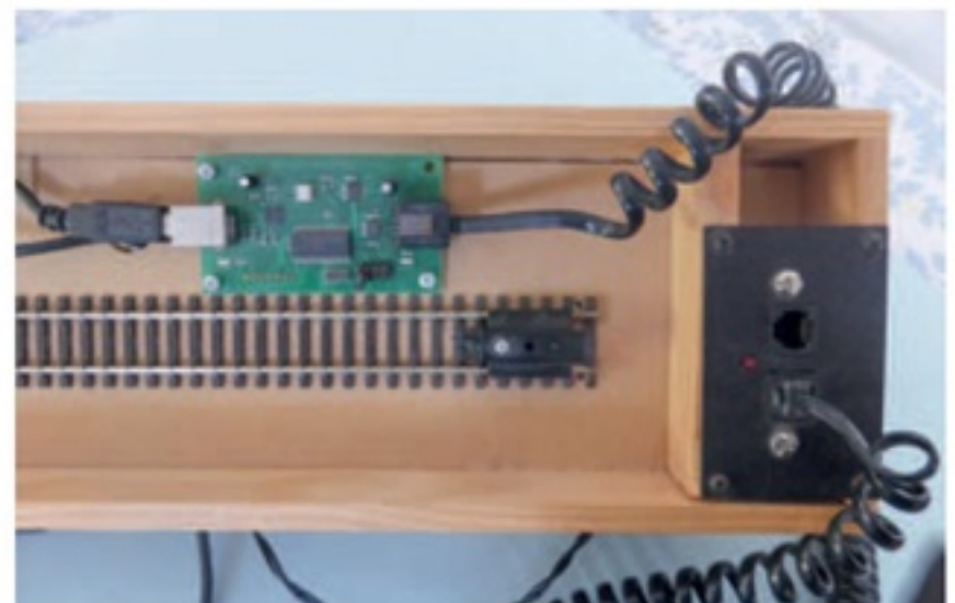
Right DCC test module. It also has a Kadee coupler height gauge installed so I can check coupler height at the same time.
