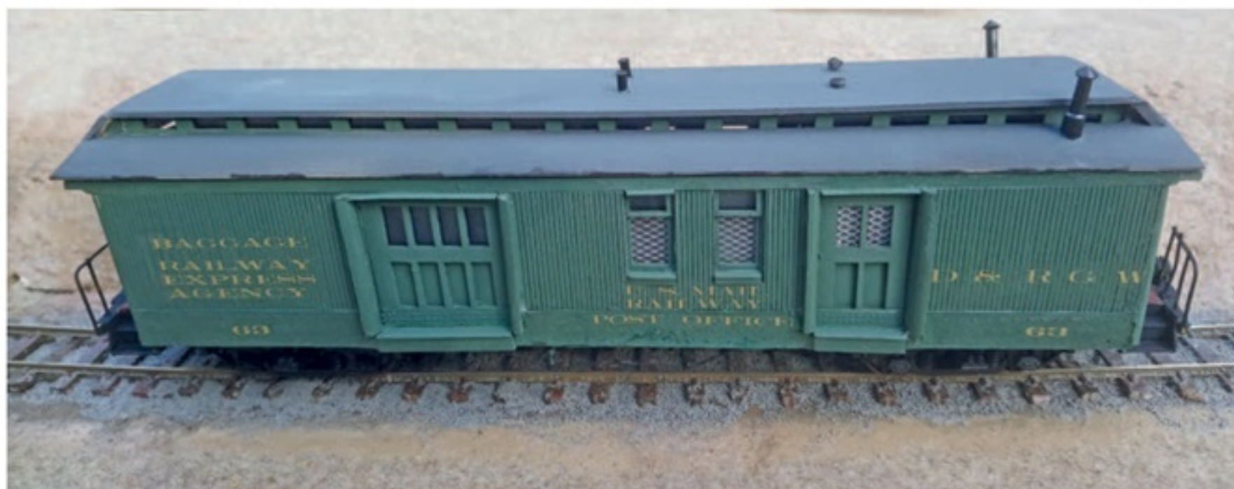
Left RPO #63 at Cerro Mesa. The lower sides of the baggage cars and RPOs were fitted with steel sheets for security. To model this effect, card was glued on and then rivet decals added.
