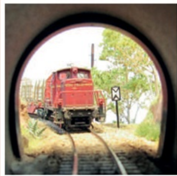
Above A V60 approaches the tunnel, passing the Vorsignaltafel for traffic in the other direction.
