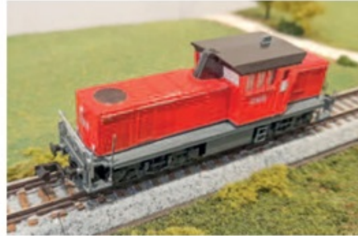
Left The Rh2068 3D-printed body and running plate compared to the Roco DB BR290.
