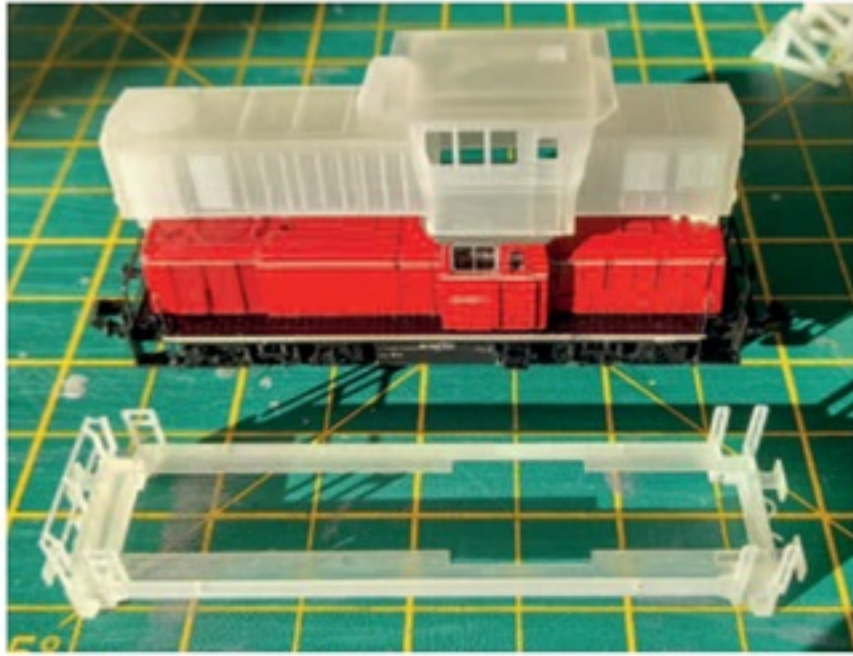
Left The Rh2068 3D-printed body and running plate compared to the Roco DB BR290.
