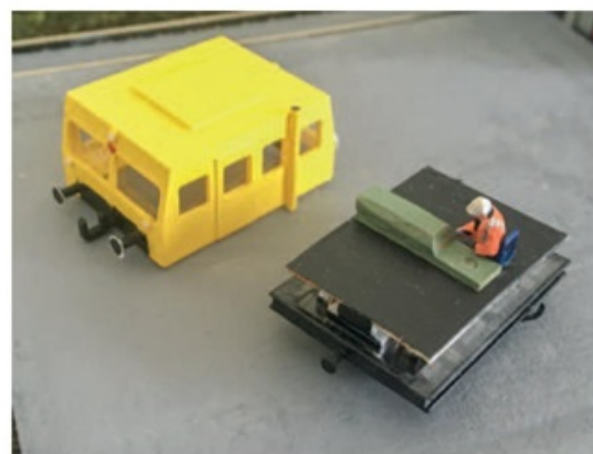
Above right The Rh2068 diesel features a 3D-printed body on a Roco DB BR290 mechanism.
