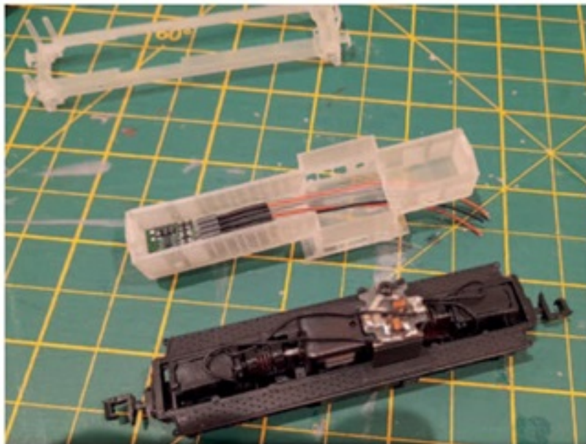
Left The DCC decoder fitted neatly inside the long hood.
