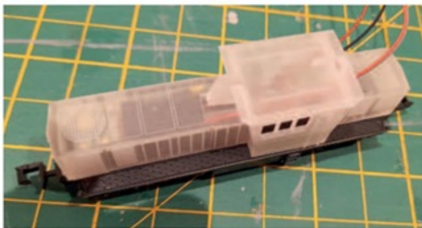
Left The body with the decoder in position in the long hood is tried on the mechanism. I later decided it would be better in the cab.
