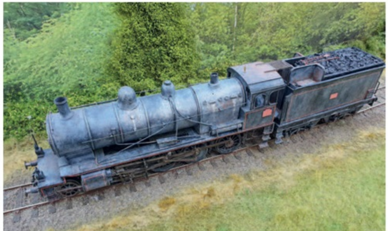
Above and below 140C 38 was the first loco to be scratchbuilt – at least in terms of the body as the chassis is from a Stanier 8F with little modification.
