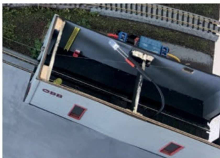
Left The necessary electronics are concealed within the buildings; the roofs can be easily removed for access.
