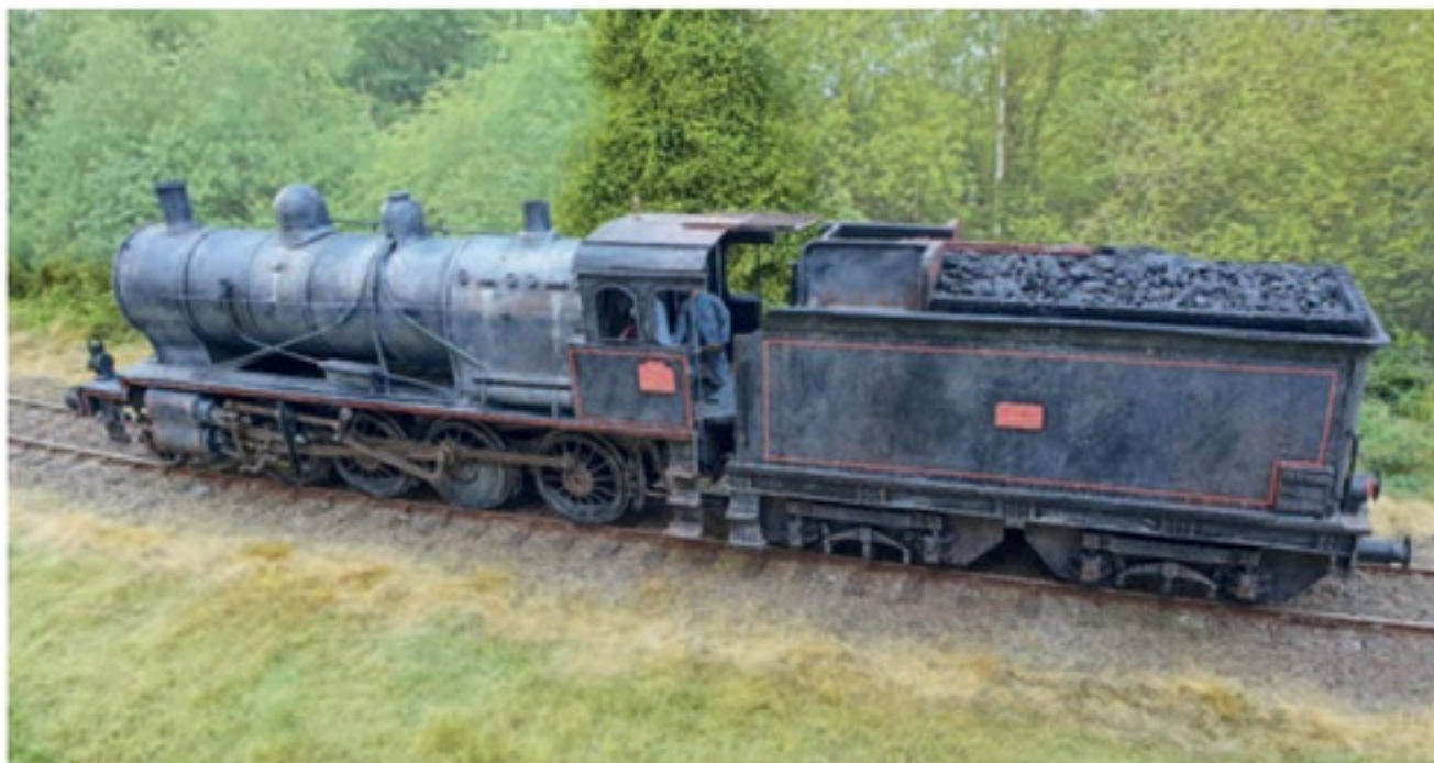
Above and below 140C 38 was the first loco to be scratchbuilt – at least in terms of the body as the chassis is from a Stanier 8F with little modification.
