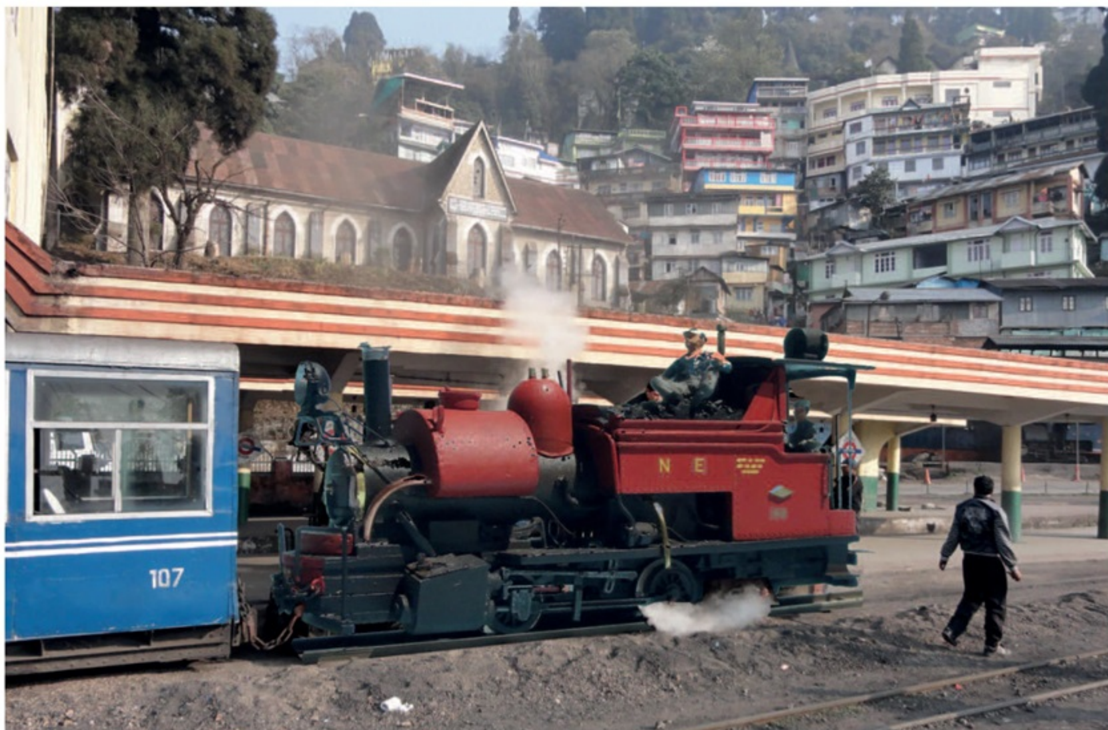
Above No.45 at Darjeeling station ready with a downhill train. The coal breaker is on the bunker, but the sanders are not required for this trip.
