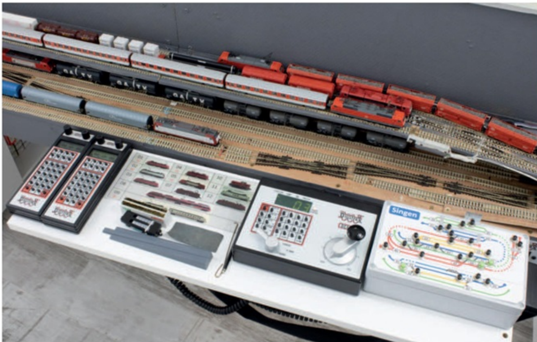
Left Behind the scenes storage and the DCC controls, with the point mimic panel on the right.
