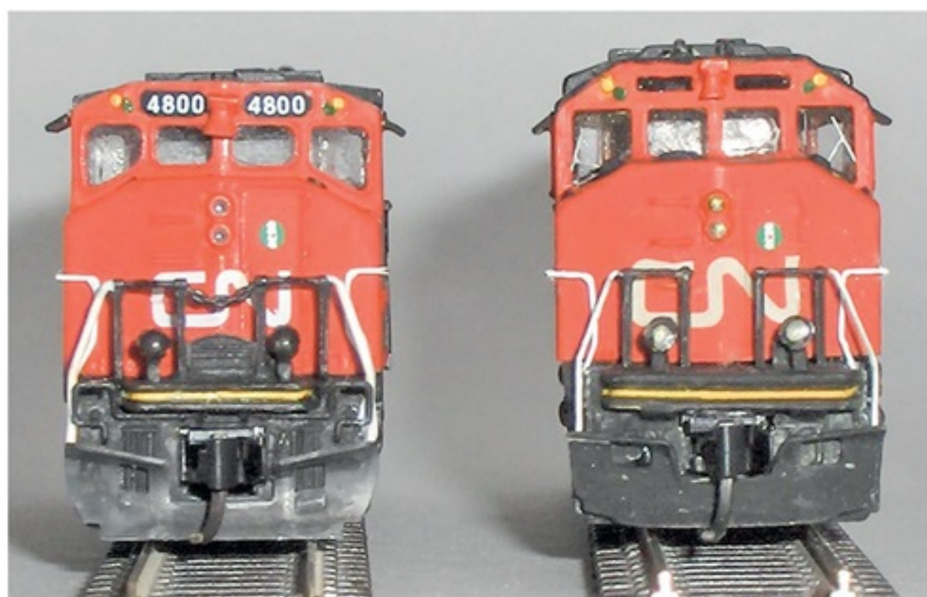
Below Comparison of comfort cabs showing anti-climbers and ditch lights.
