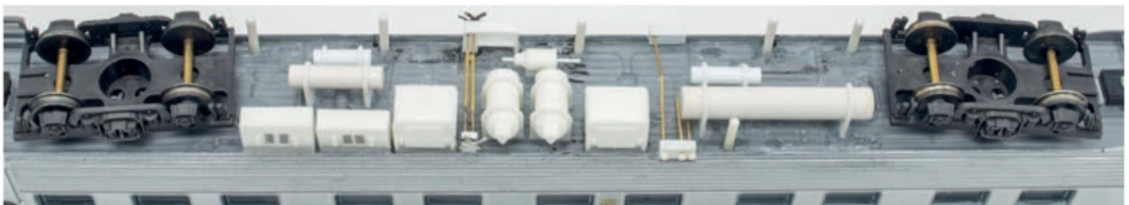
Below NAM underframe parts not yet painted: water tank and air tank at the non-door end; calorifiers, air conditioning units, and brake gear in the middle; equipment boxes and tanks at the door end.
