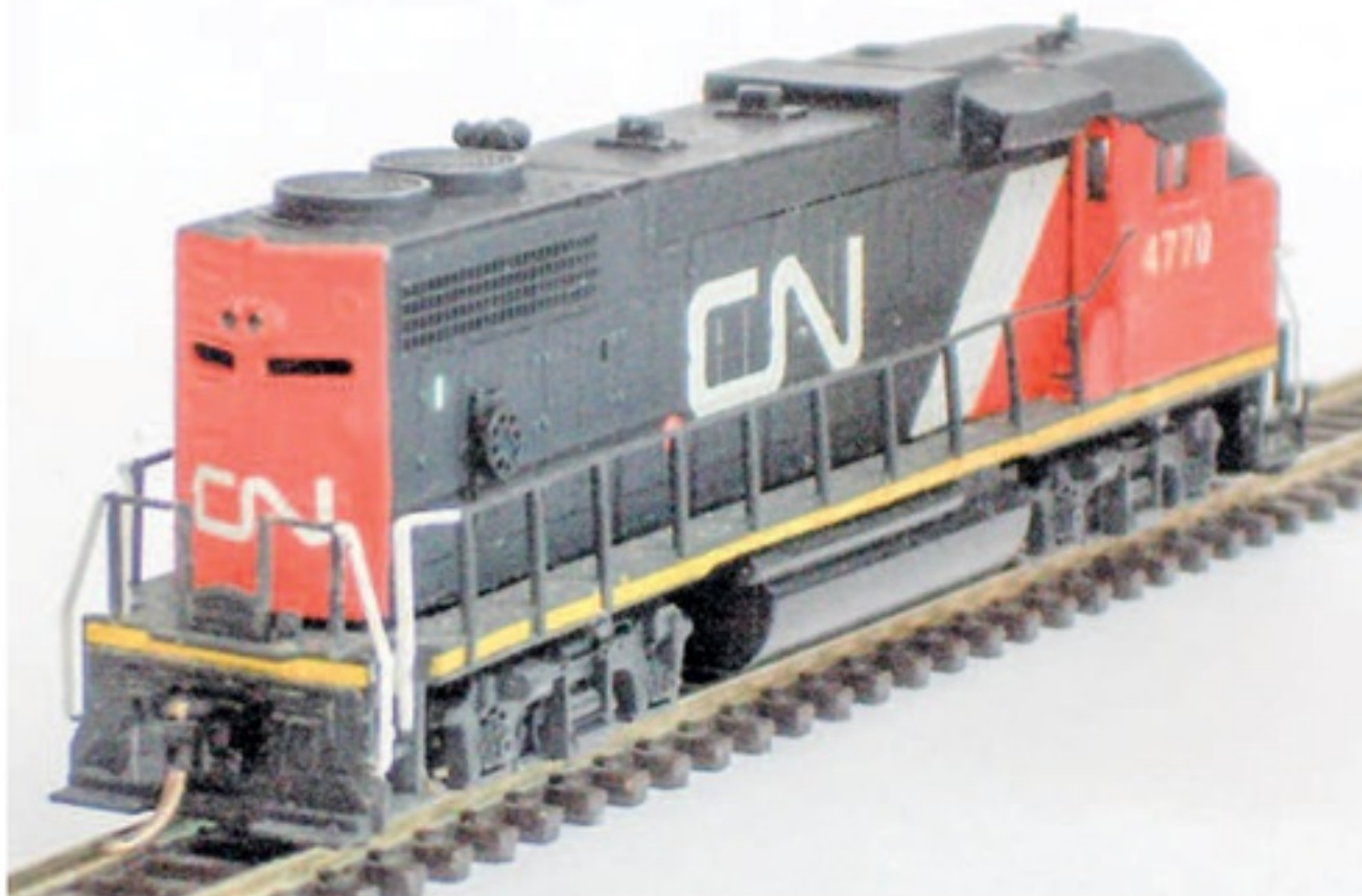
Below Rear of #4770 showing false brake handwheel recess on the side of the long hood.
