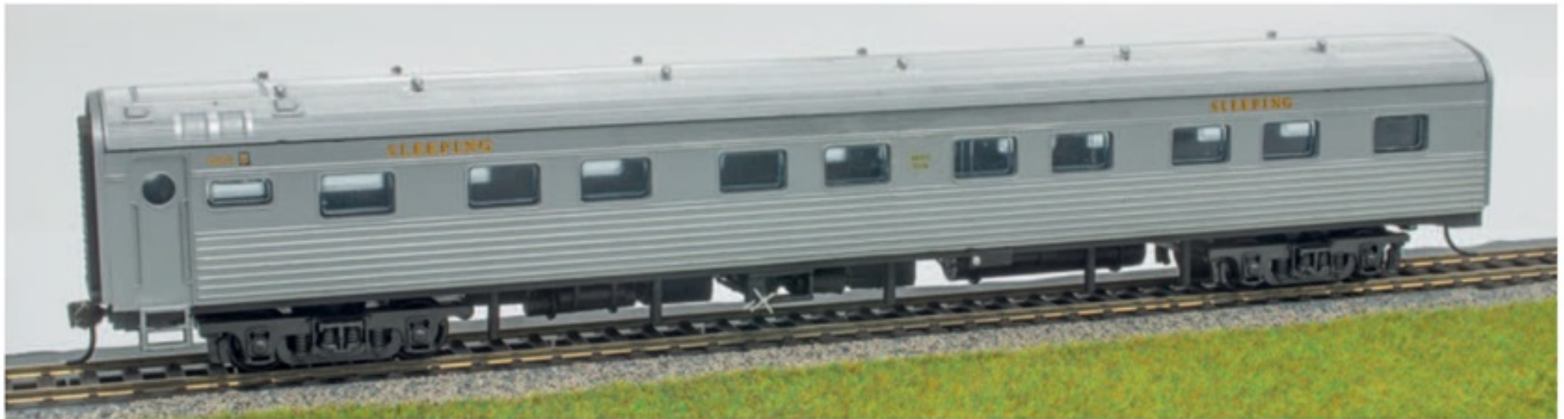
Above NAM 2336 right-hand side with torpedo vents above the compartments, shower, and toilet cubicles.
