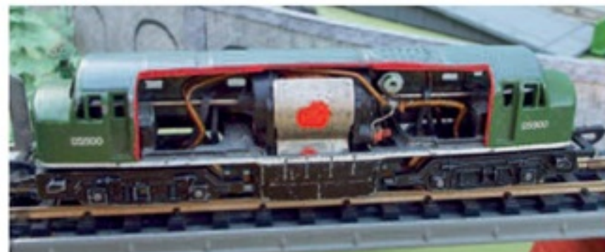
Left I modified this locomotive with the body cut away to show the original drive.
