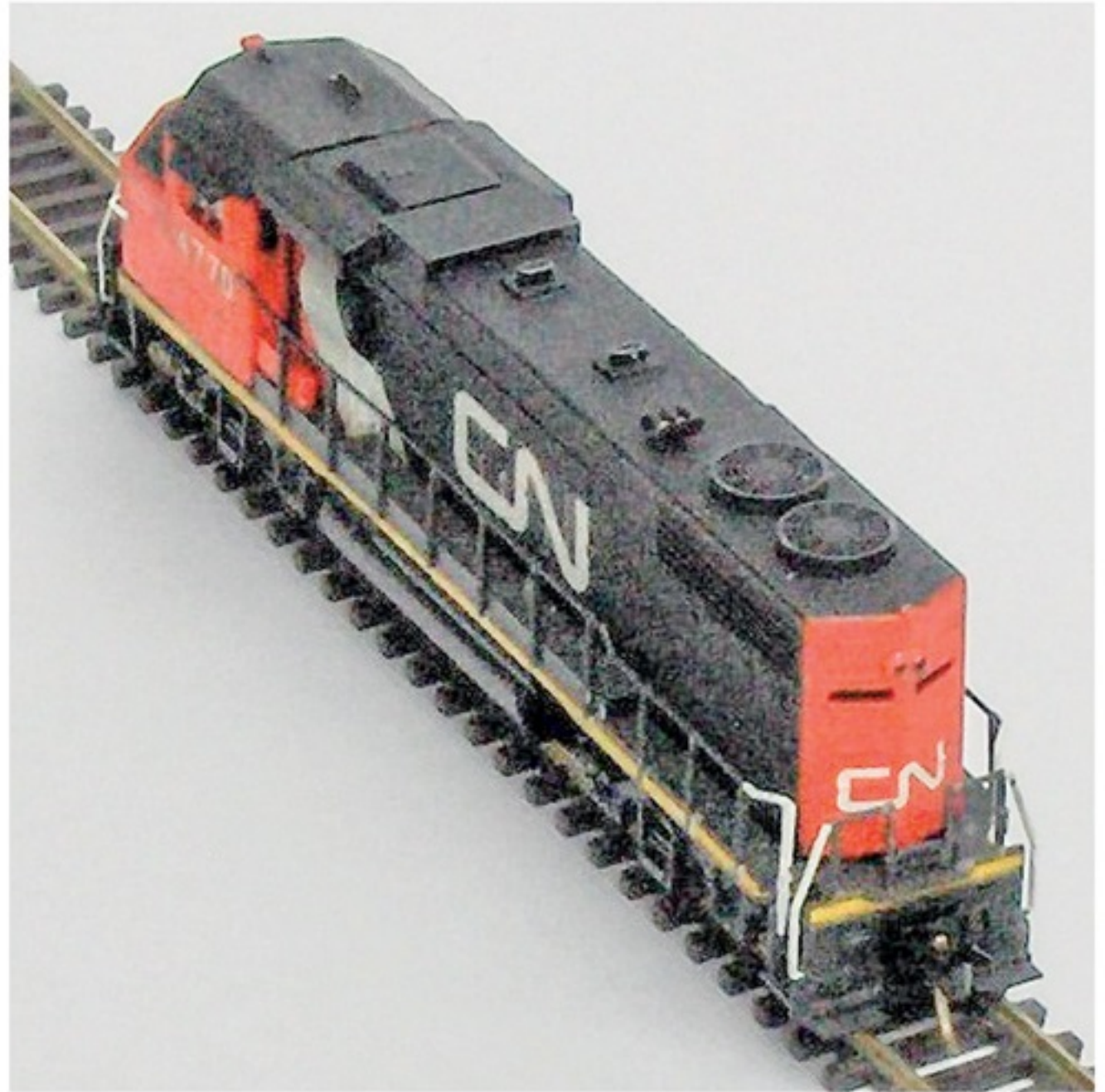
Above Long hood detail of #4770, showing repositioned horn and salvaged exhausts.
