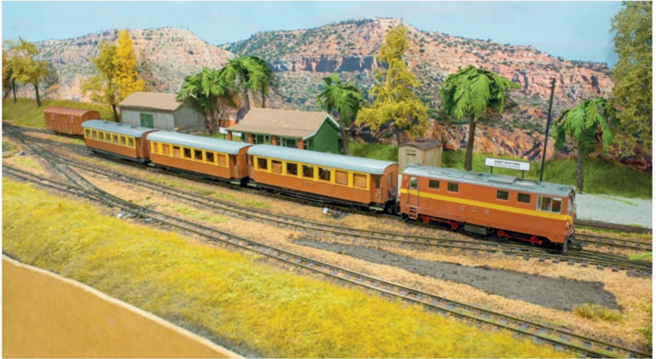
Above Modern Image on the CGR – a B-B diesel hydraulic with a train of steel-bodied Gloucester RCW coaches. The model is a repainted Roco Austrian Rh2095, and the coaches modified Liliput.
