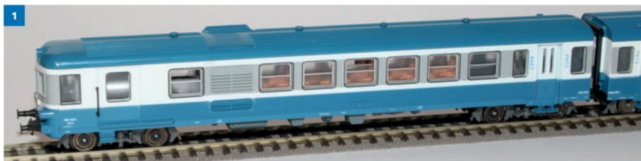
1. One of the power cars as it comes: an elegant body equipped with a classic Jouef motor bogie. Even forty years after its release, it still looks good though it does not meet current technical standards. The motor unit is camouflaged behind frosted windows.
