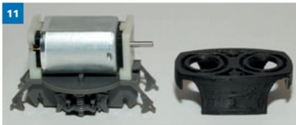
11. The new motor installed on the bogie frame, the two white L-shaped pieces being tightened in their respective places. On the right, the cap.
