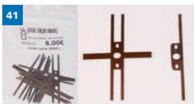
41. To provide power for the lights in the trailers, pick-ups must be fitted to the wheels. I chose a product from CDF (ref.8045810). It is necessary to cut two of the wipers in half, as the X4900 bogies have both wheels on each axle isolated by centre bushes.
