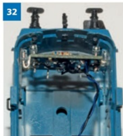
32. The PCB with the white LEDs for the headlights (characterised by a yellow dot) outside and the red tail light LEDs inside. The connection tails were bent into an S shape to obtain the exact spacing in the body.
