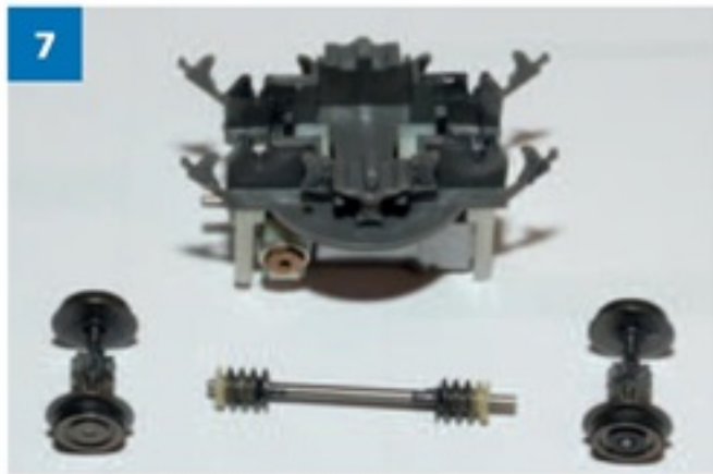
7. Underside of the original motor bogie, with the axles and the layshaft with two worms dismantled. The layshaft projects at one end to fit the gear wheel.
