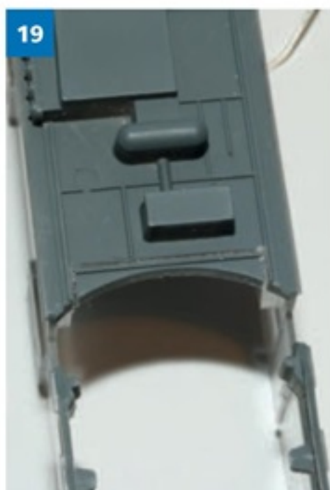
18. As this stage I realised that with the transmission gears at the front of the power bogie, as originally, it was impossible to accommodate the LEDs. So I decided to re-position the bogie with the transmission inside, that is to say toward the centre of the chassis. This meant modifying the base of the chassis: two saw cuts are visible here.
