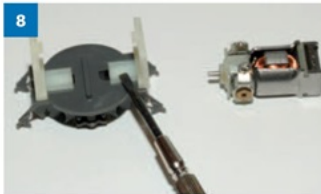
8. Top of the power bogie, with the original motor removed. To do this, one of the two white L-shaped pieces was moved using a small screwdriver.
