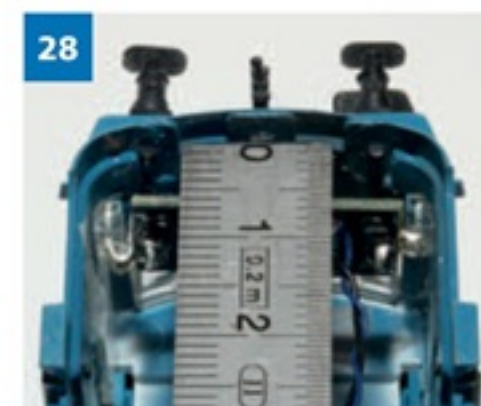
28. With the PCB held in place by the two white LEDs, a ruler was used to measure how far the red LEDs will have to protrude from the board to meet the inside of the body.
