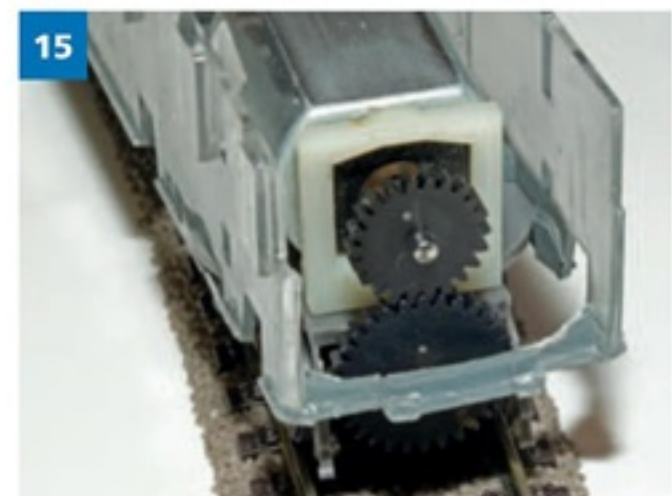
15. The modified motor bogie installed in the chassis for testing. The front of the glazing must be trimmed so that the large black transmission gear, now at the bottom, does not touch the frame.
