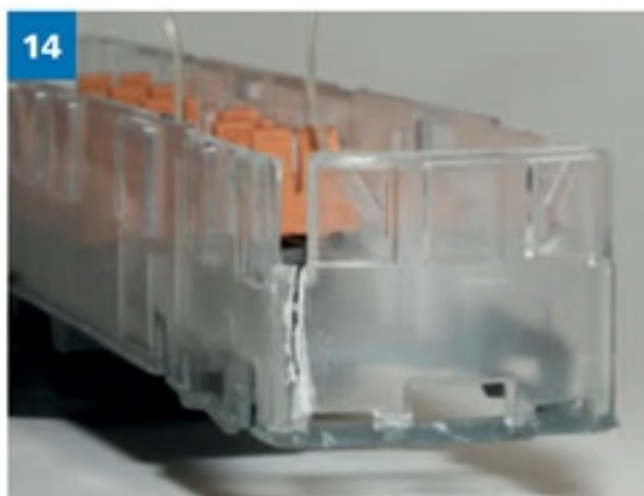
14. Modification of the glazing at the front: a vertical cut has been made to remove the front of the glazing, to recover all three panes of the windscreen.
