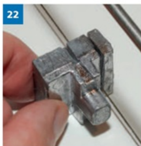
22. With the opening in the frame enlarged, the ballast weight is now too large and must be cut down on one side. I used a small modeller's saw, changing the blade twice: lead clogs and significantly wears the teeth of the saw blades!
