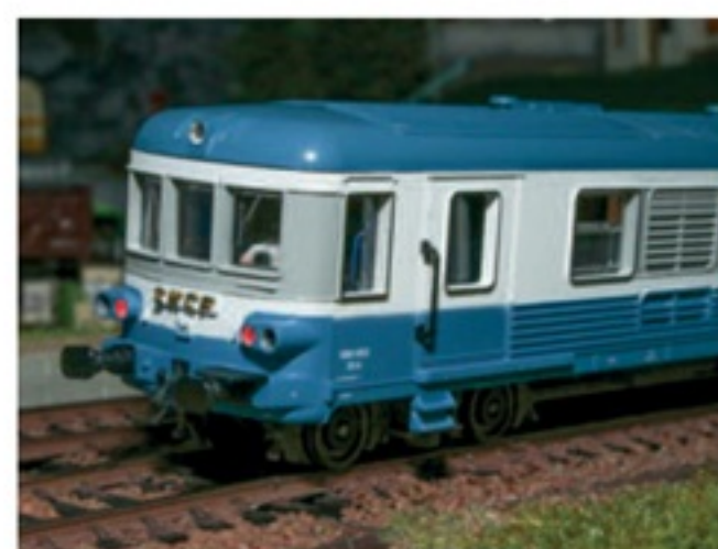
To re-assemble the X4900 the body, with lighting in the passenger section and working head and tail lights, is simply positioned on the modified frame, and pushed on little by little, until it snaps into place.
