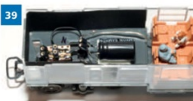
39. The anti-flicker capacitor for the interior light strip was held with double-sided tape at the rear of the chassis. It will be connected to the strip, under the roof, via a mini-connector.
