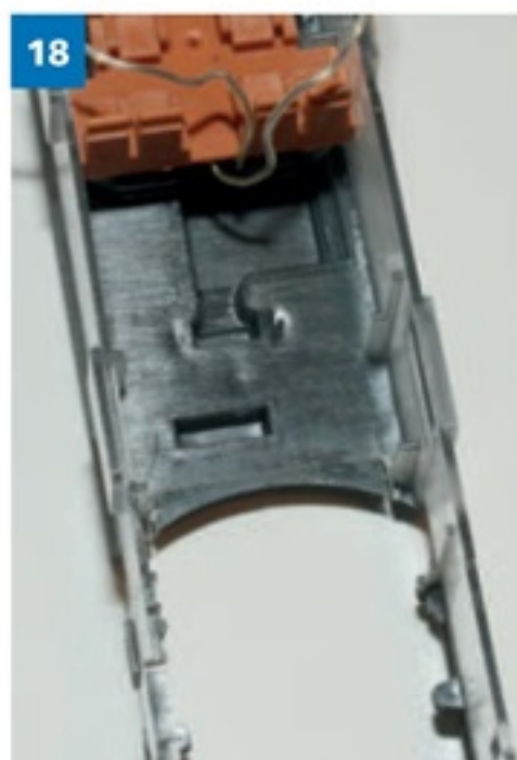
18. As this stage I realised that with the transmission gears at the front of the power bogie, as originally, it was impossible to accommodate the LEDs. So I decided to re-position the bogie with the transmission inside, that is to say toward the centre of the chassis. This meant modifying the base of the chassis: two saw cuts are visible here.
