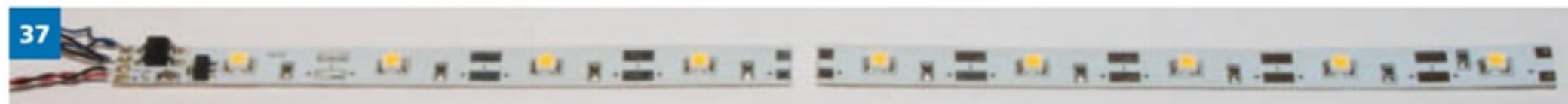
37. A lighting strip (in this case from Lapierre Modélisme or Limousin Modélisme) was fitted to illuminate the passenger section. It can be cut to length with small pattern cutting pliers. I held it in place under the roof with double-sided tape.
