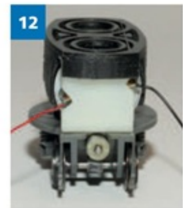
12. The front of the motor bogie, with wires soldered to the motor terminals and the cap in place to check clearance.
