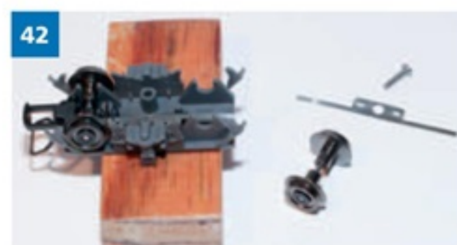
42. It is easier to install the wipers if one of the wheelsets is removed from the bogie.
