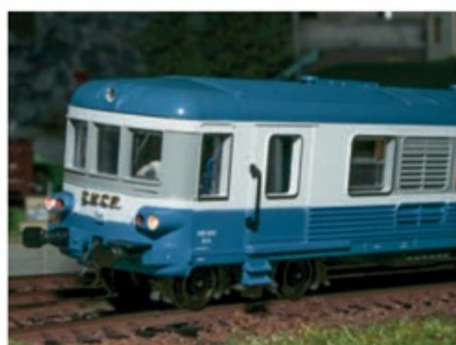
To re-assemble the X4900 the body, with lighting in the passenger section and working head and tail lights, is simply positioned on the modified frame, and pushed on little by little, until it snaps into place.
