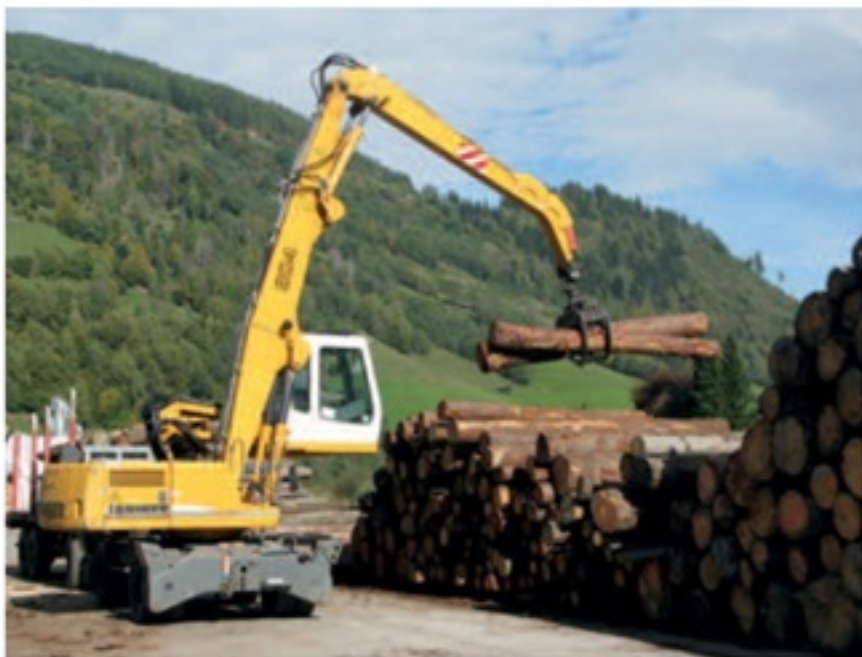
Left Moving logs from a stock pile to a trailer (just visible beyond) with a mobile grab. These machines are also used to load railway wagons.
