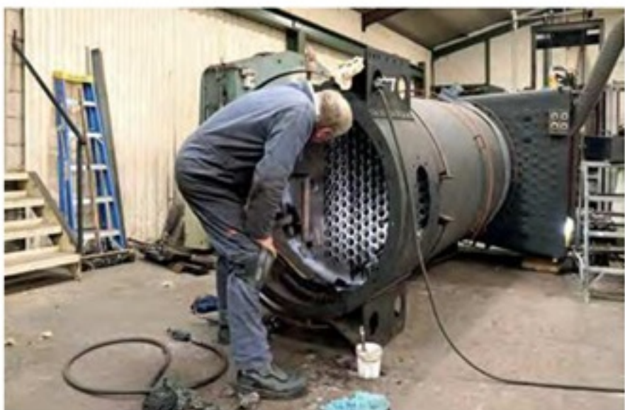
Above New tubes being fitted in the boiler shop. 20th February 2020.
