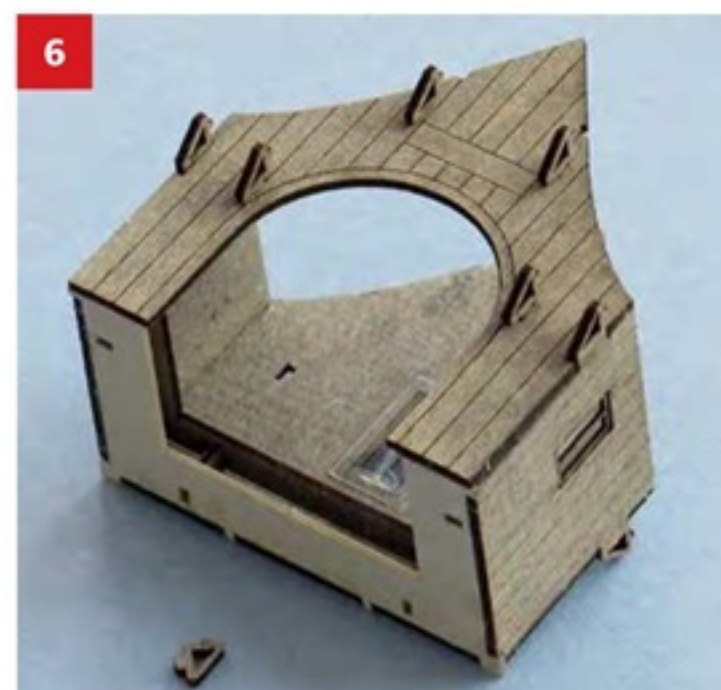
4. Two walls and the floor have been assembled, and I am now working on the other wall of the building. I used UHU Holz Leim because it is a tacky adhesive with a short drying time and so very suitable for laser-cut kits.
