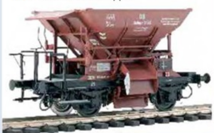
KM1 Talbot ballast hopper
