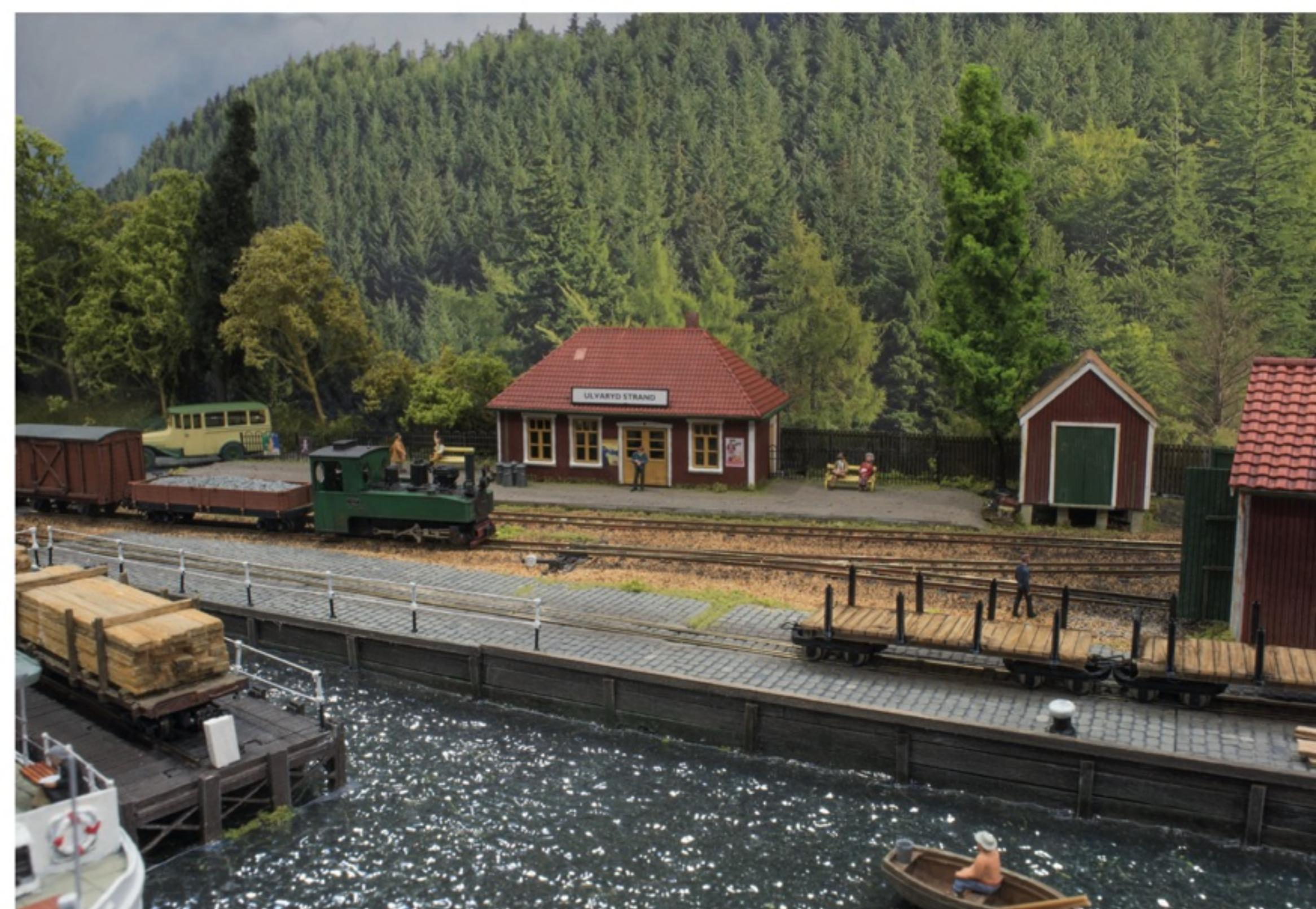
Trackwork is also boringly conventional. I used Peco OO9, with flexible track at the front and along the rear, and Setrack curves. The points (all four of them!) are Peco OO9 main line points, with the exception of the Y point. They are mechanically operated, via wire-in-tube connected to a slide switch to change the polarity of the frog.
