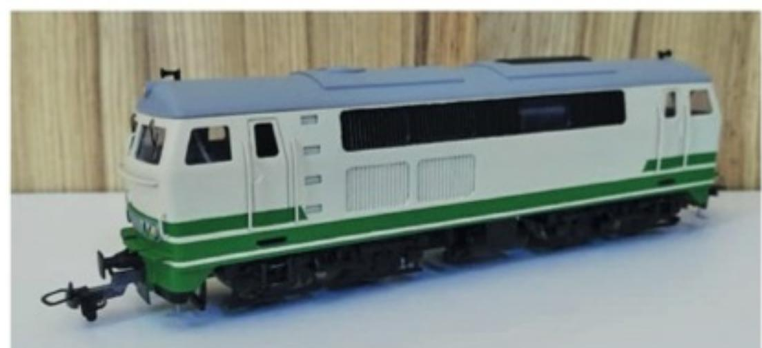
New to the Bultrains range, designed by Slav Stoyanov, is a model of the Brohltalbahn B-B diesel D5, for H0m. The body is 3D-printed (by Shapeways), with etched metal details. The model is analogue DC, fitted with a NEM 8-pin socket for a digital decoder. Price: €350.00.
