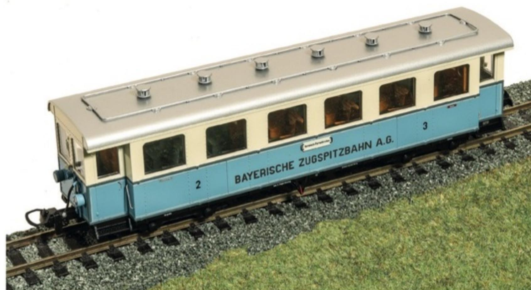
Regular narrow gauge hook and loop couplers are fitted in pockets on close-coupling mounts; imitation Scharfenbergs are supplied as optional alternatives.
