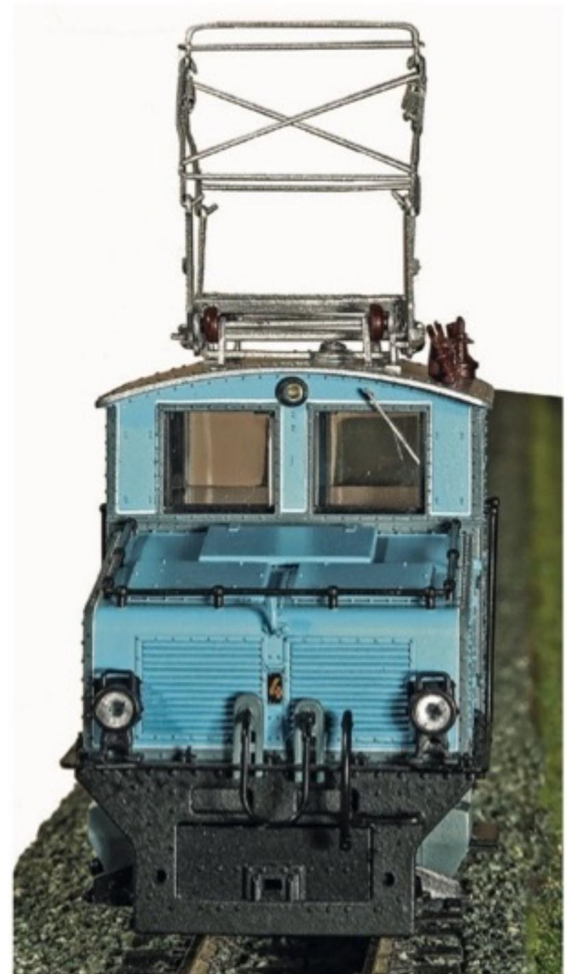
The model comes with a regular narrow gauge coupler on a flexible mount at one end and a detailed buffer beam at the other; alternative parts, including imitation Scharfenbergs, allow for equipping each end as required.
