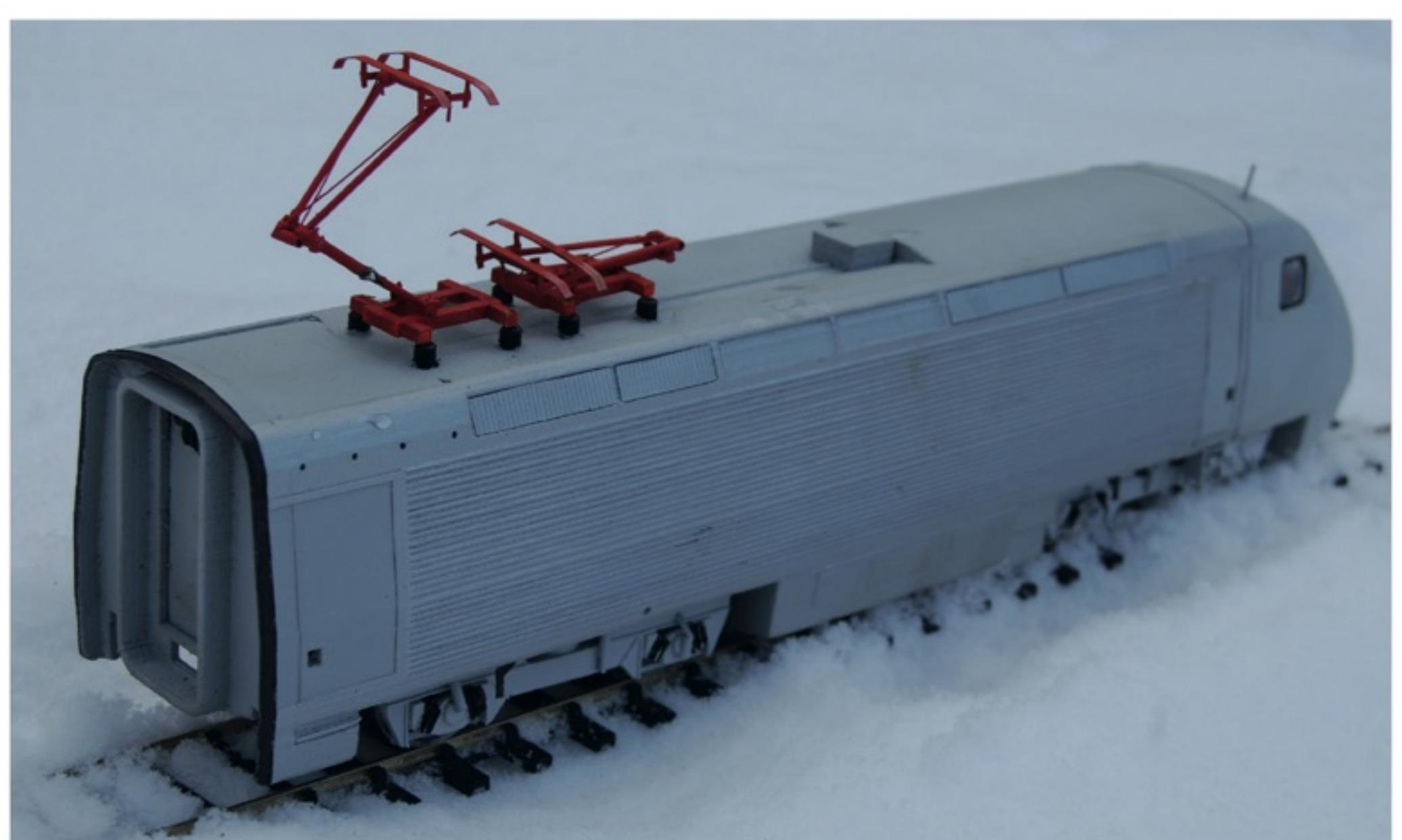
3D-printing technology is a step towards creating accurate, light, and robust body shells at a reasonable cost, if the initial design work is carried out properly. However, any illusion that a 3D-printed model can simply be taken off the printer as a finished model is far from reality. 3D-printing is a starting point, a useful tool which still requires a lot of time, effort, and skill to turn the raw print into an accurate model. But it is possible to create some stunning results.
