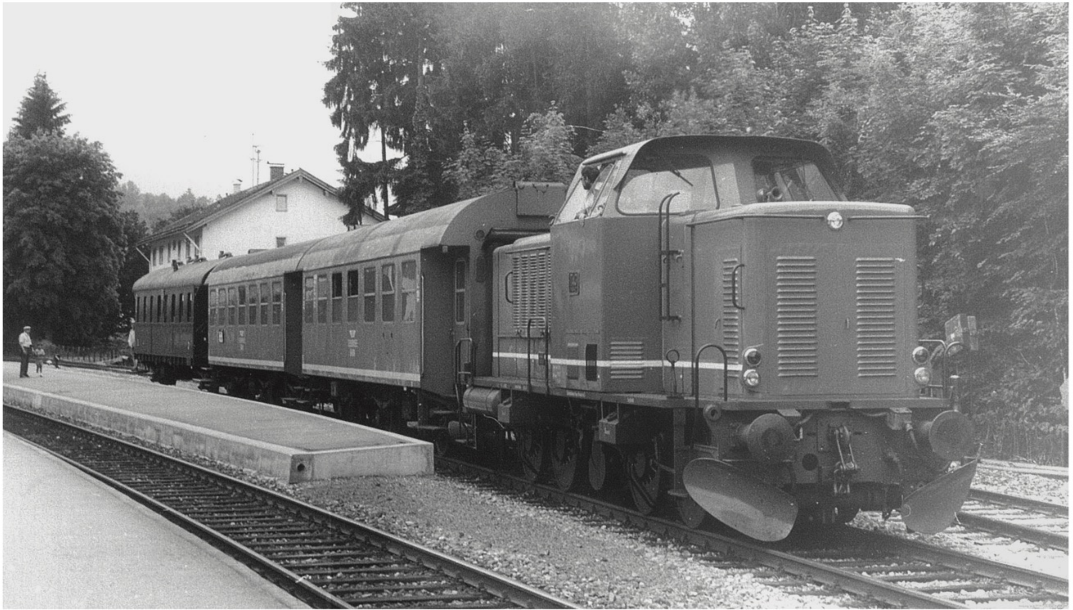
Above Tegerenseebahn MaK 0-8-0 diesel No.12 at Tegerensee on 19th June 1988 with two Umbau coaches and an old 'Thunderbox' four-wheeler. Photo: Frank Hornby.
