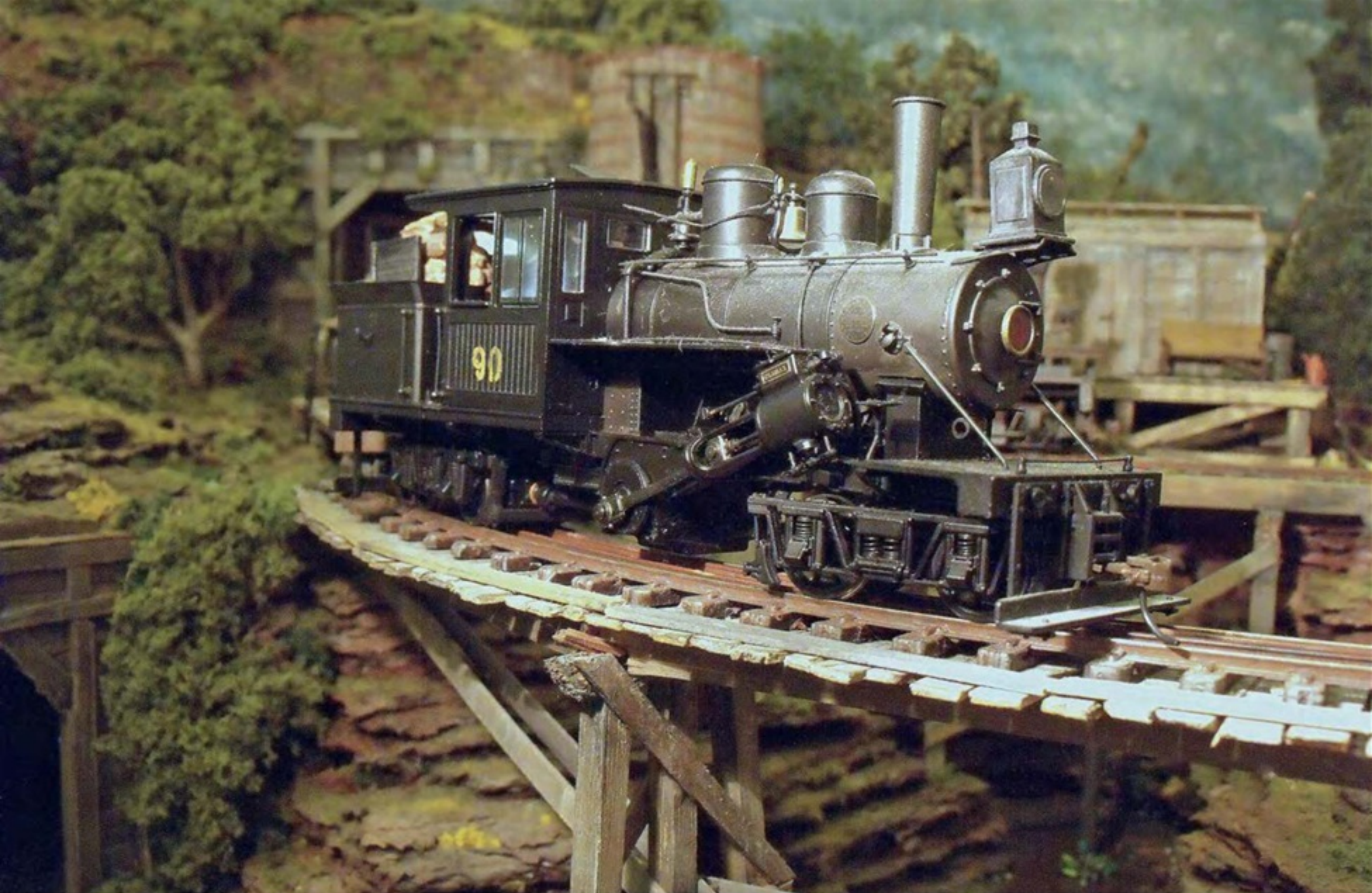
Above Geared articulated locos like Climax #90 and the Shays are ideally suited to the sharp curves, rough track, and light bridges.
