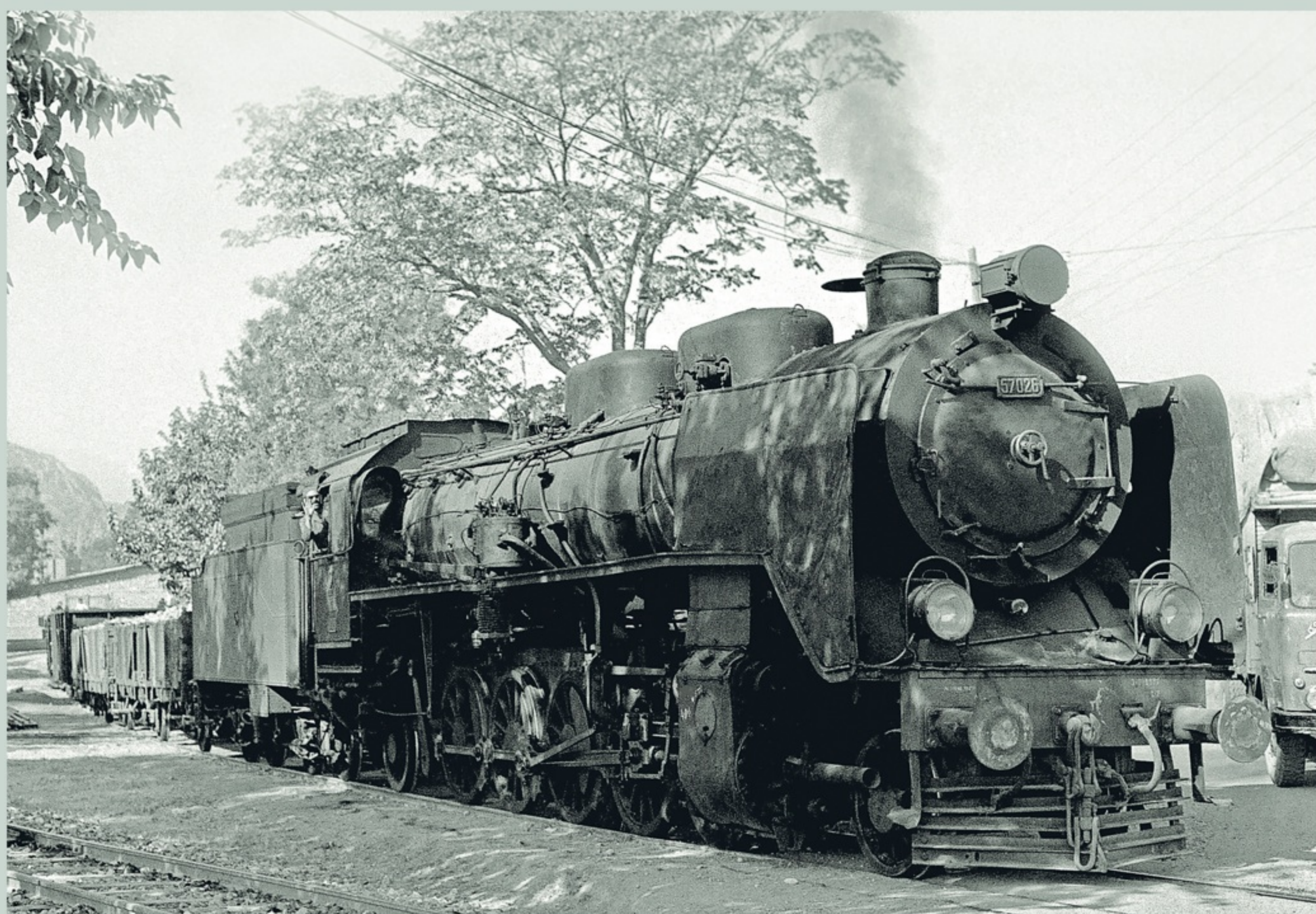
Above left G10 0-10-0 No.55013 shunts in Afyon marshalling yard. This locomotive was built by Nohab in 1928.
