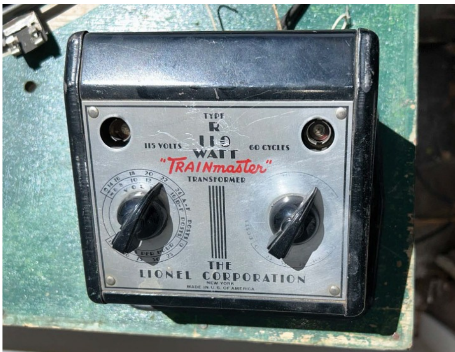
A Type-R 110-Watt Trainmaster Transformer provided enough power to operate a train and the various accessories on the SR47, including two freight loaders and a gateman.
