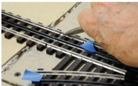
When working with track and installing plastic insulating pins, it is a good idea to mark each center rail for wiring later. Here, the author is cinching up each rail tightly for good electrical contact.
