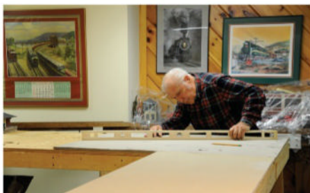
Before installing any track or switches on a layout, be sure your benchwork is perfect and level all around. Smooth trackwork depends on a good foundation.
