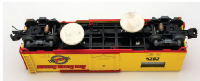
Two cleaning pads, attached to discs, rest on spring-loaded posts.
