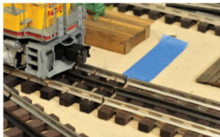
On his railroad, the author uses the middle rail on all his trackwork for signaling by gapping as shown here. Tape keeps the position of the gaps visible until everything has been wired and secured.
