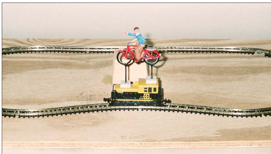
Once the bike is attached to the locomotive, connect a low-voltage DC power source to the rails and make a test run. Fine-tune it until the switcher runs smoothly.
