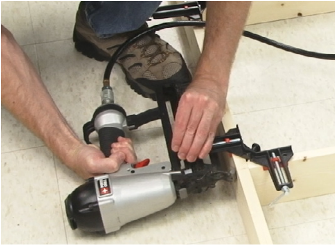
After applying wood glue to the ends, David used corner clamps and squares to align the components at a 90-degree angle. He then inserted three 2-inch brads at each joint.
