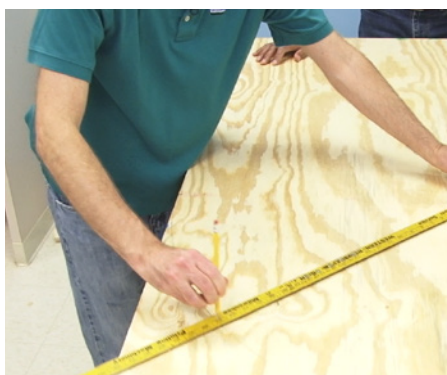
A yardstick can be turned into a compass used for tracing the rounded curve pattern.
