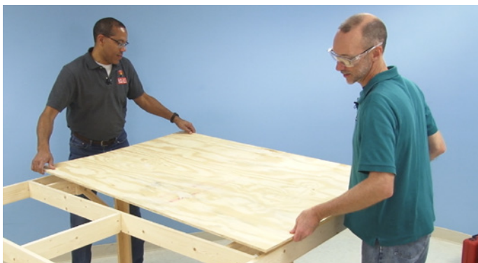
The 1/2-inch plywood used to cover the table must be cut into sections that set properly over the 1 x 4 frame components.
