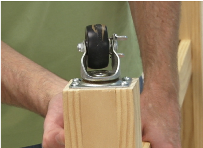
Each leg received a 2-inch caster, which will facilitate moving the layout in and around the workshop.
