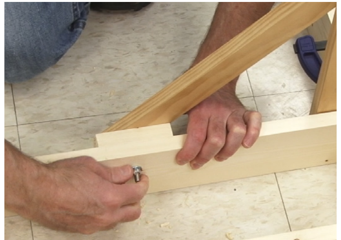
To make the layout easier to transport, David used 1/4-inch carriage bolts, washers, and nuts to make the legs removable.
