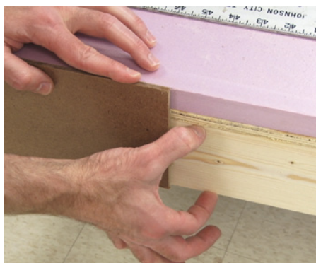
Adding hardboard fascia helps protect the foam from damage in transit.
