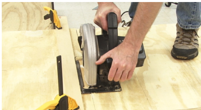
Clean and straight rip cuts can be made easily by using a circular saw and another board clamped in place as a guide.
