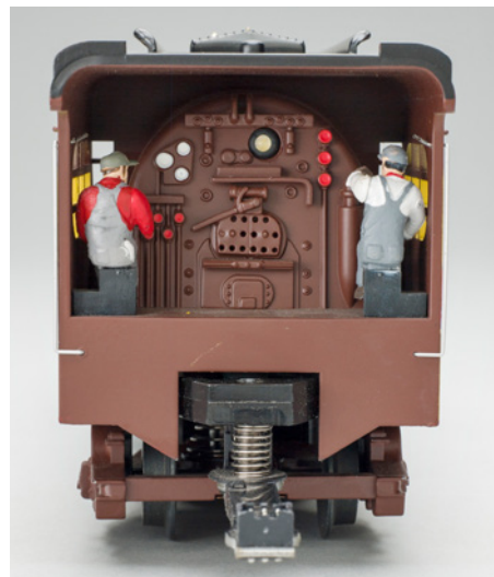
The cab has a crew, a decorated boiler backhead, painted handles and gauges, and an LED cab light.
