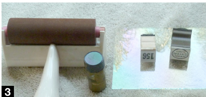
3 Robert needed to apply graphics in the Lionel style, so he obtained a rubber stamp and gold ink to practice stamping. He used the shell from an old Lionel Standard gauge no. 33 locomotive to develop his skills.
