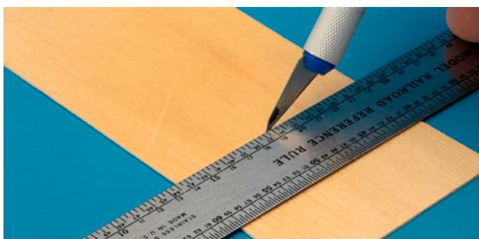
PHOTO 7. Stan used scribed hobby wood for his deck and scored a line every couple of inches to give the impression of individual boards. Adding scratches before staining shows use.
