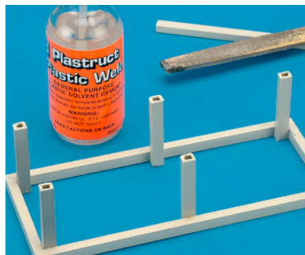
PHOTO 3. Once everything on the frame had dried, Stan was ready to add vertical supports. When installing them make sure they are square with the frame. Pressing down on each will ensure they are flush with the top of the frame.
