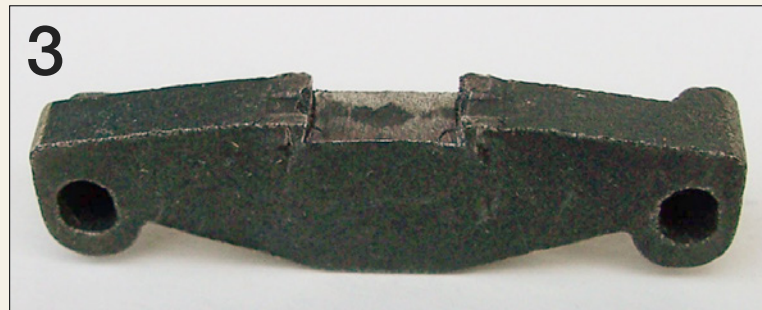
You'll need to use the files to clean broken metal or rust from the slide in the truck sideframe.
