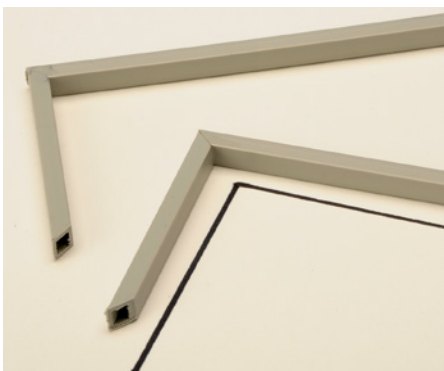
PHOTO 2. To assure a right angle while gluing the frame, Stan used a felt-tip marker and straightedge to draw a 90-degree guide on mat board. With today's fast-setting adhesives you need to hold the pieces together only briefly.
