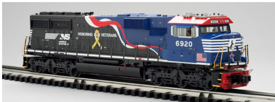
The Norfolk Southern's SD60E has a patriotic color combination. The cab's crown (top left) is a reproduction of the industry's new Positive Train Control antenna array mandated by the federal government in hopes of reducing train-to-train collisions.
