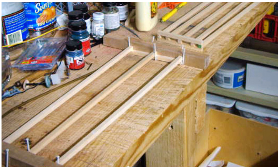
FIG 4. Finishing nails and wood blocks ensure each bent will be identical. They also serve to hold the pieces together as the carpenter's glue dries.
