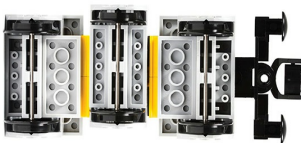
Three-axle truck with sliding middle axle, as seen from below
